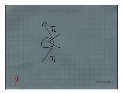
So, based on this rap angle if this is T 1 the T 1 and T 2 are related with friction and the rap angle, invariably T 2 may be high in this case, where our case is different the yarn is not just passing over something called a disc it is also twisting and also simultaneously untwisting, at one area it twist in the other area it untwist. If twisting means increase in tension untwisting should mean opposite of that right.
