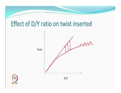
And what would we learned was that the D and Y ratio essentially, has is related with the twist being inserted into the yarn. And this twist insertion is not linear and so, there are slips as you keep on move increasing the D and Y ratio.
