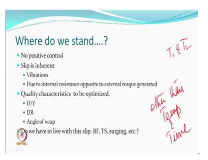
So, where do we stand we stand now saying that there is no positive control in the friction texturing and slip is inherent, because of vibrations which will happen whenever you run a machine, or it may be because of the internal resistance which is equal and opposite to the external torque. The more you twist the more is the internal resistance. So, whenever two opposing forces work, there can be slip which is surging is what we talked about.
