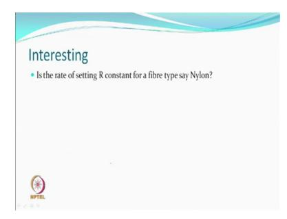
If this question is asked that is the rate of setting R constant for a fiber type let us say nylon is a constant like a specific heat is a constant, we can; obviously, say it is not constant because based on the temperature, based on the POY the residual draw ratio of the POY and even denier and so on so forth these values will keep changing and therefore, it is not constant it is only relative value based on your own material and your own specifications.
