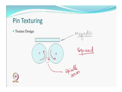
So, this is a pin or a spindle and this is spindle arm of the twister, but the twister is the whole assembly. So, your spindle is twisted and the twister assembly has this arm is resting on to disks. So, one disc moves, the other disc moves and because of that the spindle arm also moves. So, like we said last time that well it rotates at the same rpm the pin and the same rpm would be of the yarn at that particular point.
