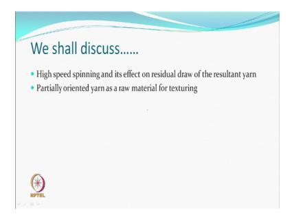
We will try to see if we use high speed spinning we said the last time we were using fibers being spun at around 500 to 700 meters per minute. If, instead of that we use high speed spinning what happens to the residual draw of a resultant yarn. And also the yarn that is produced, which is not fully oriented not fully drawn, but probably has been oriented more how does it behave for the purpose of texturing. So, looking at simultaneous draw texturing with a POY called a Partially Oriented Yarn.
