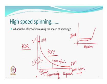
If we increase the speed of spinning alright and plot spinning speed versus residual draw ratio. Residual draw ratio means, that if you have an undrawn yarn for example, whatever and you were trying to work and then this finally, takes up the shape.
