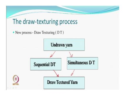
So its a new process which was; obviously, different than what people are done before. So, you can take an undrawn yarn go through a process called sequential drawing. That means, you take an undrawn yarn have a drawing unit on the machine. And after it has been fully drawn then you texturize it and then that will be called a draw textured yarn.
