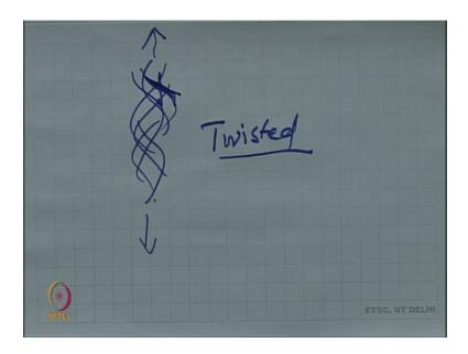
When you say you are increasing tension you are increasing the tension in a twisted yarn. What we mean is if the fiber is lying like this the tension is in this direction. And therefore, the orientation in the direction of the fiber axis is not going to be high. So, we started from the beginning itself texturing is a disorienting process. A large number of elements are lying on a twisted yarn obliquely they are not obviously, parallel to the yarn axis is not parallel to fiber axis.
