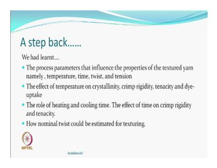
Effect of temperature on crystallinity crimp rigidity tenacity dye uptake we have seen. Role of heating and cooling time and the effect of time on crimp rigidity tenacity. And how one calculate a nominal twist just a thumb rule before you start optimizing as to how much twist is required. So, you work about twist continuing with that. (Refer Slide Time: 01:13)
