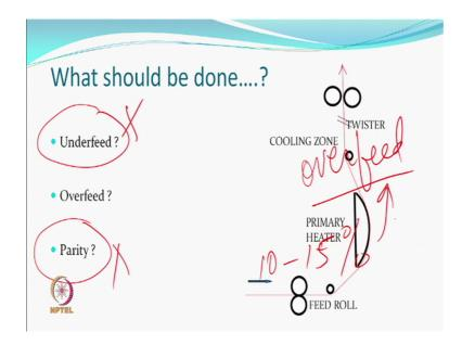
So, once we have understood the effect of tension during texturing what should we do? We have a control on the feed roller and take up roller what we do underfeed overfeed or run at parity; that means, the speeds are same.
