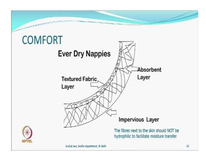
So, generally for comfort point of view and the hygiene point of view a product which we call as an ever dry nappy material which is next to skin is absolutely hydrophobic. And you could actually have polypropylene textured material as a fabric. Fabric made from polypropylene textured material I said polypropylene because supposed to have zero moisture regain.
