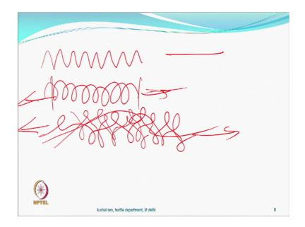
We should be able to, we can do things like this a filament instead of remaining a straight filament you can make it give some kind of crimp you can make structures of this type which are helical in nature and not flat. You may be able to introduce loops of this kind and then if you stretch any one of these they will extend. And when they extend you will feel that the material at a very low stress has become very long.
