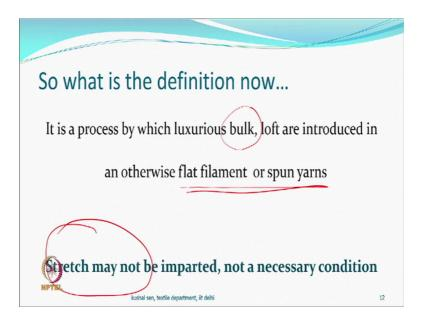
It maybe a process where definitely bulk is going to be increased right. So, bulk will be increased so we talk about bulk. So, bulk is there, but they can be flat filaments or spun yarns and also they may not have stretch. So, you can have applications where a lot of bulk has been developed, but they do not stretch. Let me just give just one small thing, this stretch is different than the elongation of a fibre elongation at break of any fibre or filament.
