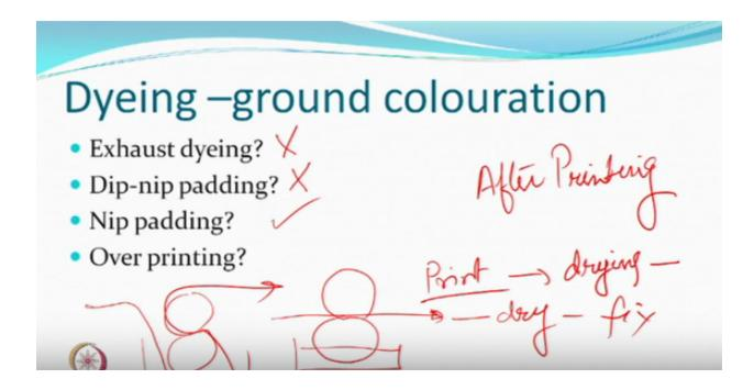
Finally, we have done the printing and after that we have to do the dyeing, which dyeing method, would we like to use, after printing. Right? This is after printing. So, we have done the printing, drying and then, we have to put the dye, first of all
