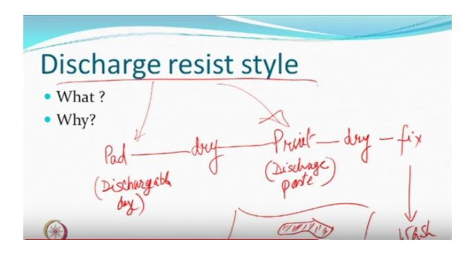
So, there's another style which is, typical for hydrophobic fibers, which is called a, 'Discharge Resist Style'. What it means basically is that, the fabric has not been dyed and fixed. So, in the earlier case what we said, that you can die, either by exhaust method or you can die
