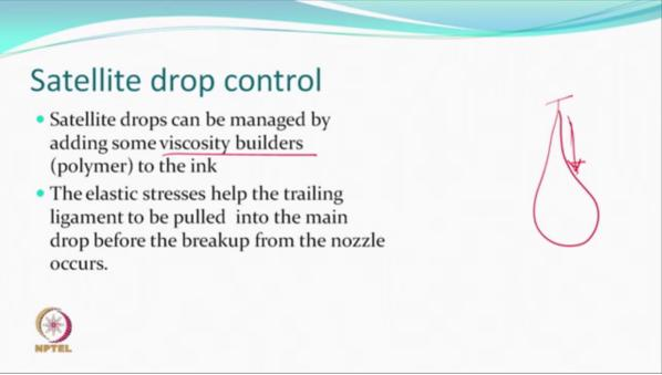
So why does it happen? So because of this small little increase in the viscosity, there are elastic stresses, which help this trailing ligament to be pulled back, okay, to pull to the drop itself and before breaking up from the nozzle. So this is one way the ink manufacturer would like to control which definitely will help in the quality of the print produced.
