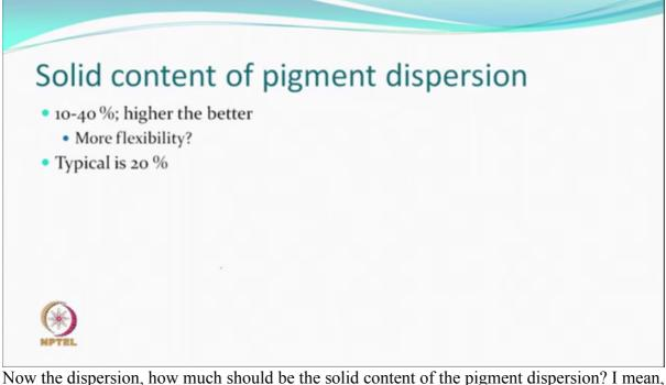
Now the dispersion, how much should be the solid content of the pigment dispersion? I mean, one can have dispersions percentage varying from 10 to 40%. Higher is the solid content, better for transport and this dispersion finally is going to be mixed with solvents, co-solvents, surfactants, viscosity modifiers. It gives you more flexibility because the concentration is going to be only diluted. Well, typically, you may get surfactants with the dispersions and solid content of about 20% or so.
