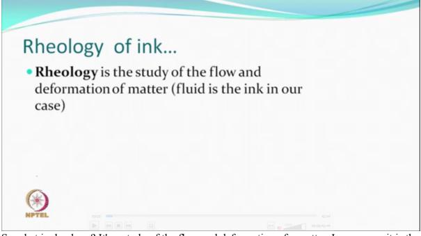
So what is rheology? It's a study of the flow and deformation of a matter. In our case, it is the ink, which is flowing through a nozzle.
