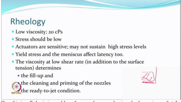
Here this is called priming and here there can be some cleaning also happening so that the next time when it goes for the printing to the other direction, the jetting is very nice. So it is always in a ready to jet condition.
