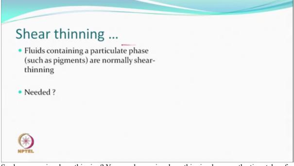
So do we require shear thinning? Yes, we do require shear thinning because the time taken for even the smallest droplet to come out of the nozzle is very, very small and therefore rate is very high. And so if it is not there, there will be back pressure develop. The actuators may not work very nicely. They may get affected adversely. Their functions may be really affected badly and so we do require shear thinning behavior of the inks for printing.
