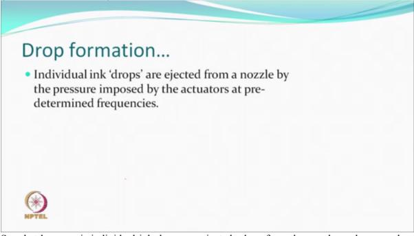
So what happens is individual ink drops are ejected, okay, from the nozzle, and you apply a pressure and the pressure is by various actuators add frequency, which are predetermined, like we already probably know that the DOD type of machines or systems require less frequency compared to the CIJ types, and so based on that frequency, there are going to be pulses, which are going to be ejecting the drops.
