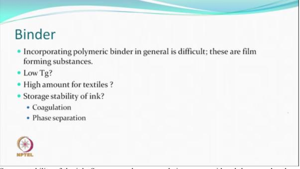
Storage stability of the ink. So one may have coagulation as we said and there can be phase separation between things which are very soluble in water versus which are less soluble in water. All that can cause a problem and binders, therefore, prove to be more difficult ingredient.
