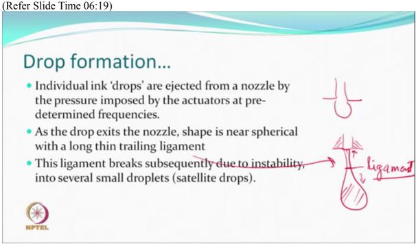
We expect that the ligament breaks subsequently due to instability because there is gravitational force and the push which is taking it away, and then it may, while it is breaking,
