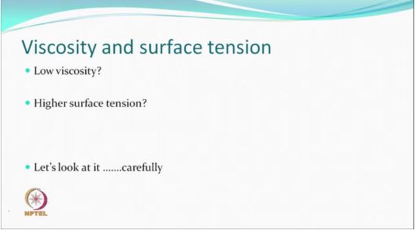
In general, the viscosity and surface tension are going to play an important role. You can appreciate that the inks which we use for inkjet printing are low viscosity systems. If it was a very high viscosity system, then, obviously, it will not pass through, unlike, for example, our conventional printing.
