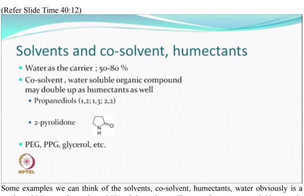
Some examples we can think of the solvents, co-solvent, humectants, water obviously is a carrier which may form about 80% of the volume. The co-solvent, water soluble organic compounds may also double up as humectants as well. That would means you will have to add less amount of material, for example, we just said propanediols or pyrolidones and polyethylene glycol, polypropylene glycol, glycerol etc., may form another group of chemicals to be added.
