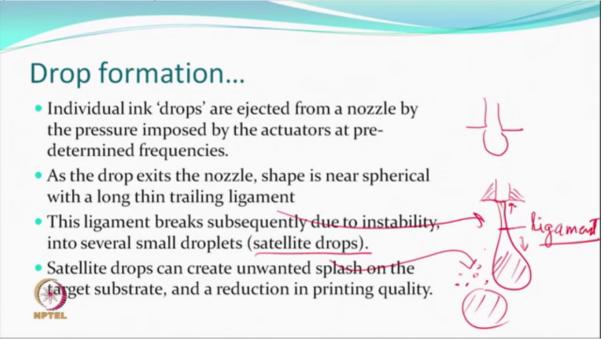
I don't think it's a good idea. Satellite drops can create unwanted splash on the target substrate, whether it's a paper or a fabric, and this obviously means there is a reduction in print quality.
