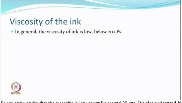
So we again revise that the viscosity is low generally around 20 cps. We also understand if viscosity is too high, clogging and other things can happen, and we also understood that even at this low viscosity, the rheology profile cannot be ignored and it is controlled with relatively high molecular weight water-soluble polymers.
