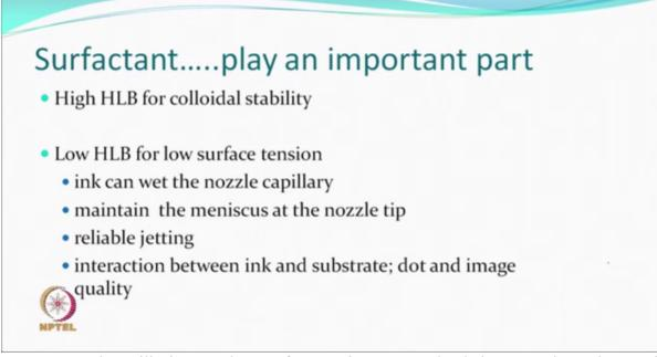
Low HLB value will give you low surface tension. It can also help you to keep the nozzle capillary always wet. It can also help to maintain meniscus at the nozzle tip and it can also be reliable jetting and as we said before that interaction between ink and substrate can also be affected. Dot and image quality, both of them are so important to us.
