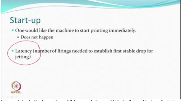
Latency is basically the number of firings needed to establish the first stable drop for jetting. If something is sticking somewhere, some portion is dried up, the holes are not really clean, so it takes how many firings it is required before everything smooth comes out is called latency and this is what sometimes known as start-up issues.
