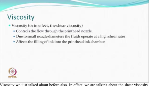
Viscosity we just talked about before also. In effect, we are talking about the shear viscosity. So it controls the flow through the printhead nozzle. Due to small nozzle diameters, you can understand so many of the nozzles are there in very small area. The fluid actually while it is coming out operates at a higher shear rates.
