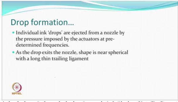
And as the drop exits the nozzle, the shape is near spherical with a long thin trailing ligament. For example, if this is the exit of the nozzle, the drop initially may come like this. As it moves further, so it may actually have a spherical thing with something which is extending we are calling as the ligament.
