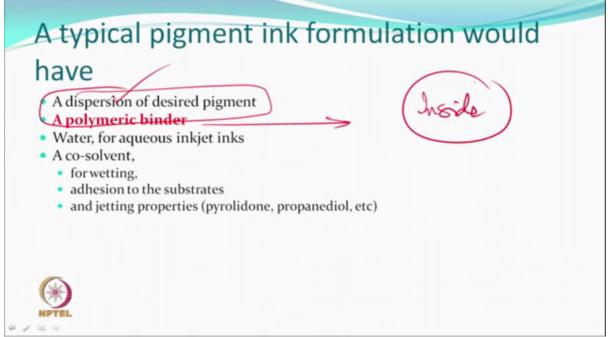
A co-solvent so that the surface tension and wetting properties are modified to suit the requirement. It will have the purpose of wetting, adhesion to the substrate and good jetting. Some of the examples which compound which can be used are pyrolidones or propanediols etc.
