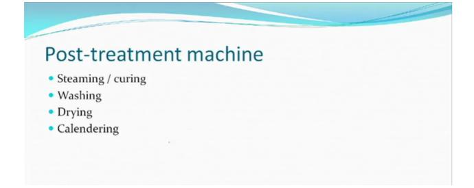
Post treatment, as we said, would have steaming, curing, washing, drying, calendering and then, based on what type of a color that you have. Steaming with etcetera, for reactive, acids curing for pigments, washing of course if required and drying, calendering, these are the simple treatment that you, anyway would like to do. So, we can stop here and next time we'll, talk about, Inks.
