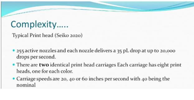
So, complexity in one of the typical examples, like this particular print head, which is made by Seiko called two zero two zero. for example, has something like 255 active nozzles, you know, nozzles may be more, let's say, the shared wall so you may, ensure that only one of the side one, starts the other one is not firing. So, all of them fire then, there could be something different, so you may have active and all this
