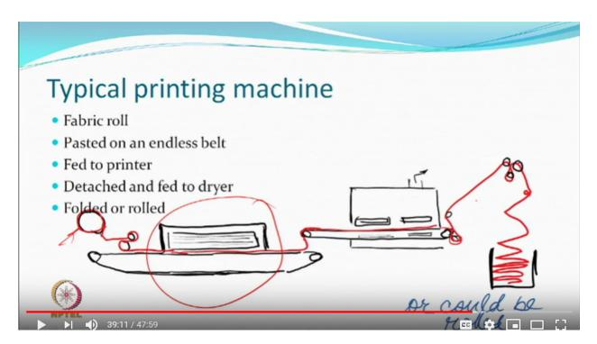
So a typical fabric machine, printing machine, may be looking similar to what we have seen somewhere, so you have a fabric roll, then you have an endless belt, where after some controlled, stretching and pushing, you apply, a fixit here, it moves in the print head, get sprinted and then, you take it on top, dry so
