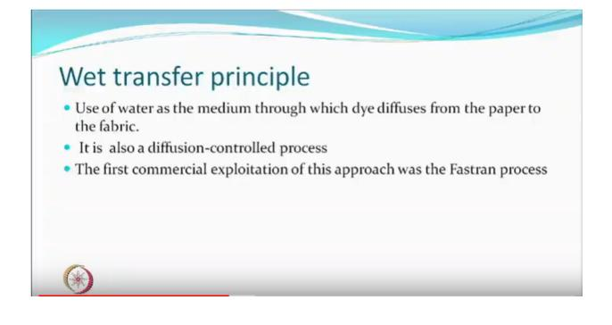
So, the principle basically remains the same, but the medium is no water, because, you are now talking, about hydrophilic material, which is the fabric and so, you have similar mechanism, as you looking at any other printing mechanism. So, diffusion control process and one of the processes, which was commercialized was called the,' Fast Tran Process'.
