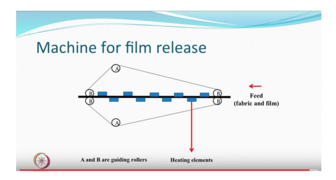
So, simple sequences, of this type where there are many heating elements, along the surface or some kind of a blanket, which is forcing, the paper and the fabric together and one can hopefully, get the transfer or release of the film from the paper. So, the whole thing the printed element printed part can come out.
