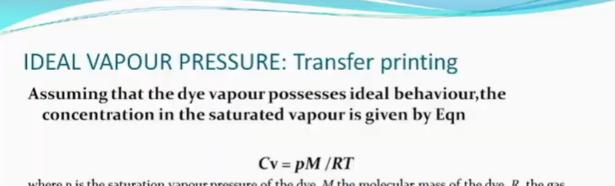
where *p* is the saturation vapour pressure of the dye, *M* the molecular mass of the dye, *R*, the gas constant and *T* the Temperature.
