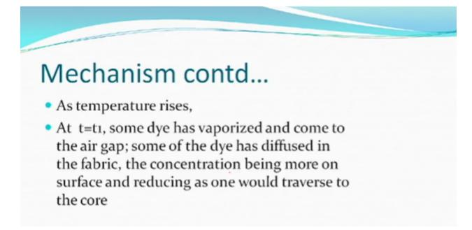
And the temperature rises, some dye has vaporized, has come to the air gap, some who died has diffused in the fiber, the concentration being more on the surface and reducing as one would Traverse to the core the fiber. So, this is what we said that the concentration will be more, on the surface of the fiber, as you go inside the fiber, the concentration of dye will be less, something similar is here. Refer Slide Time :( 26: 51)
