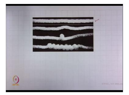
So this is the actual yarn, actual twisted yarn. What we do? We put in the twist tester and we try to increase the twist of the yarn. After a few rotations, what you will see is that you will see this kind of image. So the axis of the yarn will not be straight first. It will happen gradually. First it will be straight almost straight. Then, the axis deviates from linearity significantly. After a few insertions, you will suddenly see that the structure collapses.
