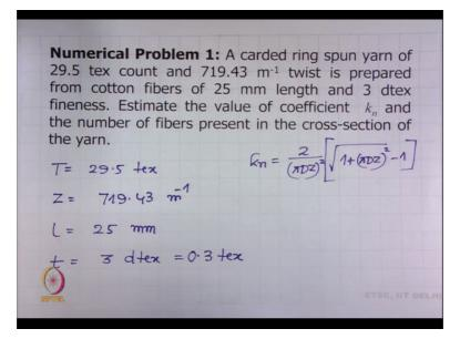
A carded ring spun yarn of 29.5 tex and 719.43 twist is prepared from cotton fibres of 25 millimeter length and 3 decitex fineness. Estimate the value of coefficient kn and the number of fibres present in the cross-section of the yarn. This you have to solve. How will you solve this problem? Now what is coefficient kn? Coefficient kn we have learned using helical model. The coefficient kn is 2/pi D z square square root 1+pi D z square-1.
