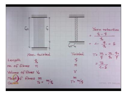
This is a parallel fibre bundle or non-twisted fibre bundle. So let us write here non-twisted bundle and this is the result after twisting. So this is twisted bundle. Now these two bundles, non-twisted as well as twisted they have certain characteristics. Let us establish those characteristics first. The first characteristic is length. What is the length of this bundle is zeta 0. What is the length of this twisted bundle?
