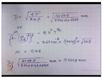
Yarn diameter is 4T/pi mu rho. That is your yarn diameter, T is given. What is T? 4\*T is your 29.5 tex/3.14, mu is not given and it is a cotton fibre this millimeter. So mu is not given, how will you find out mu? Mu you have to come back to your module 3 in order to find out mu. You remember this formula in module 1, module 3. Now Q carded ring spun yarn 9.61\*10 to the power -8.
