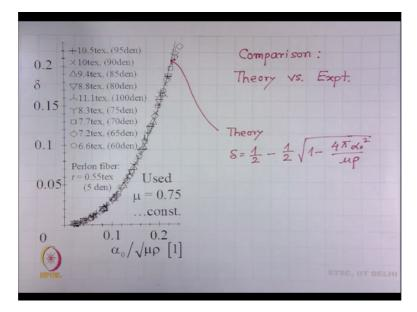
Theory versus experiment, a lot of yarns were studied and along the x axis alpha 0/square root of mu\*rho is plotted, along the y axis retraction is plotted and all these points are basically the experimental results for different yarns and this line you see, there is a continuous thin line going on, that is basically coming from theory. What is this line? You have just now derived root over 1-4 pi alpha square/mu\*rho right.
