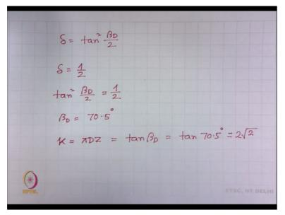
And we have already found out that tan square beta D/2 and if the limit of retraction is 1/2, so tan square beta D/2 is=1/2. Then, what will be beta D? Beta D will be 70.5 degree. That means the twist angle of surface fibre there is a limit and that limit is 70.5 right and then what is your twist intensity? Twist intensity is pi D z that is equal to tangent of beta D. Now if you substitute tangent of this what you will find out? 2 root 2.
