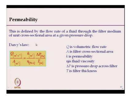
Another important characteristics is the permeability. This is defined by the flow rate of a fluid through the filter medium of unit cross-sectional area at a given pressure drop.
