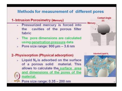
There are different types of porometer. First is that intrusion porometry that is mercury intrusion porometry. This method is where mercury is used, pressurized mercury is forced into the cavities of the porous filter fabric. So, this is the cavity. Here the mercury
