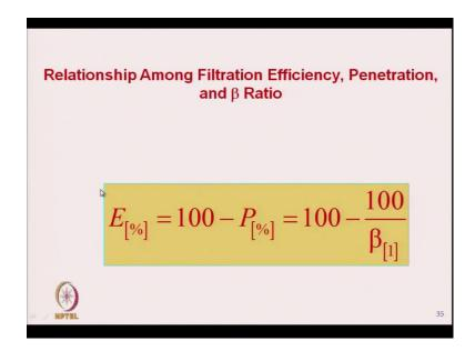
This is the relationship between filtration efficiency, penetration percent and beta ratio.
