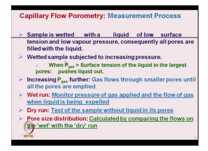
So, the process is that sample is wetted with the liquid of lower surface tension; sample is first wetted. And low vapour pressure consequently all pores are filled with the liquid. So, initially the pressure is measured and the liquid is wetting the total surface ok.
