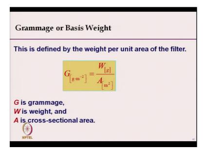
Now, we will discuss the physical properties of filter fabric. First is that grammage. This is simple mass per unit area, its nothing special in it here mass of fabric in gram and take the area. And we calculate the mass per unit area that is expressed either in terms of basis weight or grammage. In filter fabric, we use that term grammage or basis weight very commonly ok.
