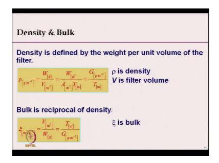
Next is density and bulk. And density is defined by the weight per unit volume of filter and density its this is W is a weight and volume V. And from there, if we actually the replace volume with cross sectional area and the thickness that will be G is the grammage; the mass per unit area W by A by thickness. So, density we can get from mass per unit area and thickness. So, we can calculate the mass per unit area and we can
