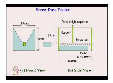
Now, the screw type dust feeders are used normally this is stepper motor connected with the screw rod ok. And here its a front view; this is a side view. Once this motor rotates at known speed, constant speed due to the screw system, the dust from the hopper is flowing through this horizontal side from left to right. And here at the exit point, this is actually feeding the dust in the vertical pipe. And the flow rate of dust or dust feed rate can be changed by changing the speed of the motor.
