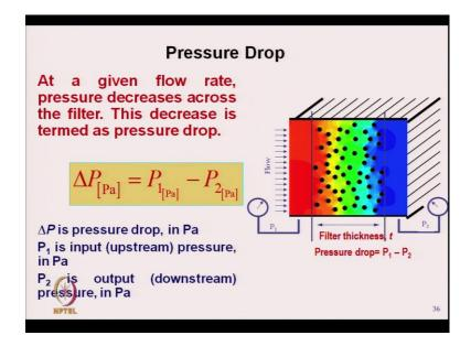
Another important parameter for filtration which is pressure drop. At a given flow rate the pressure decreases across the filter. This decrease is termed as pressure drop. So, when the particle along with the liquid medium flows across the filter media, so this is the flow direction, this is upstream, other side its downstream. So, in upstream side, we have very high pressure and as its flowing through the filter media and then other side there will be lower pressure.
