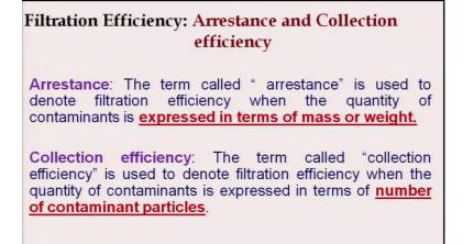
This filtration efficiency can be expressed in two ways; one is arrestance and another is collection efficiency. Typically this two terminologies are actually filtration efficiency. So, arrestance the term we used when we express the contaminant quantity in terms of mass or weight. The term called arrestance is used to denote the filtration efficiency when the quantity of contaminants is expressed in terms of mass or weight.
