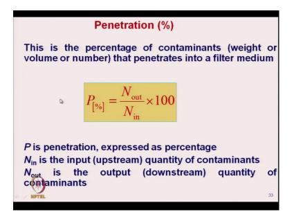
So, in earlier case, in penetration efficiency, it was Nout/Nin, it may be in terms of weight volume or number. But in beta ratio, this is the ratio
