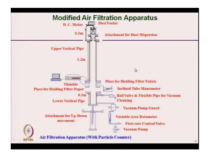
So, here this total system is connected here; its controlled by the software. And the data of the filtration efficiency and the dust free data are captured. These are the particle counters. Here you have the particle counter at the upstream side and another is the
