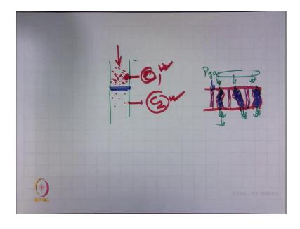
But in this system this measurement system, this is the vertical orientation of pipe, here we have the filter medium. And the dust particles are coming this is in upstream direction; and after that this is down downstream direction. And here we have put one, counter 1, here we are putting counter 2 and this particle counters will count the number of particles per unit volume of air.
