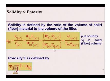
Solidity and porosity; so, what is solidity? Solidity is defined by the ratio of volume of solid that is the fiber material to the volume of filter that is total material filter. So, it is expressed in terms of  $\mu$ , volume of fiber by volume of filter medium.
