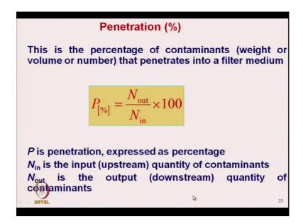
And in terms of penetration percent, so this penetration percent this is the percentage of contaminants that is weight or volume or number that penetrates into the filter medium. So, penetration percentage is
