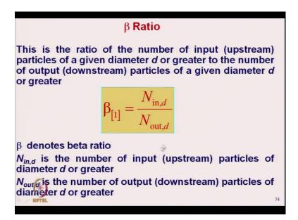
And beta ratio, this is the ratio of number of input that is upstream particle.
