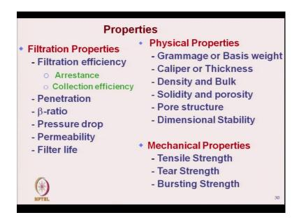
So, the properties are there three different sections of filtration properties. So, the filter fabrics are mainly meant for filtration. So, the filtration properties are extremely important and along with that there are other properties, these are physical properties. And for having proper service life, there is another property which is mechanical property. So, all three properties are important.
