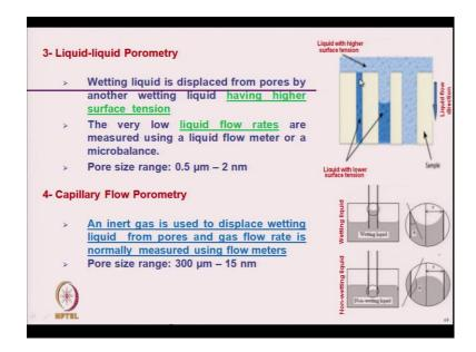
Third technique is liquid-liquid porometry. Just the name implies here we can use two different liquids. In this picture, two liquids are shown; one is in dark color; here this dark color is the liquid with lower surface tension. These are the liquid with lower
