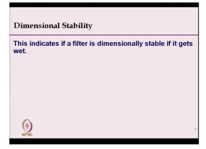
And another parameter physical parameter its a dimensional stability which is important. And when the filter gets wet, its dimension changes, so accordingly we can calculate the dimensional stability. So, we will stop here. In next class we will start mechanical properties and other aspects of filtration parameters.
