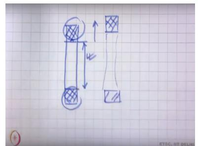
Now let us see, suppose this is our fabric specimen now what we do, we use top jaws we have gripped here at the top and at the bottom. What will gauge length? Gauge length will be actually the actual length of the specimens under the test. So, we do not consider the total fabric length this is the specimen length and gauge length is less than that is the gauge length that is the original length of the material and between the jaws.
