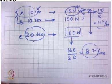
One textile material, say of 10tex has strength 100N, now another material of coarser material has 20 tex it has got the strength of 160N ok. Now how can we compare if another if yarn of 10 tex has strength of say 110 N then we can say among these two yarn we A, B, C between A and B, so this A is stronger that we see but if we want to compare A and C which one is stronger here the complexity is that it is of different linear densities.
