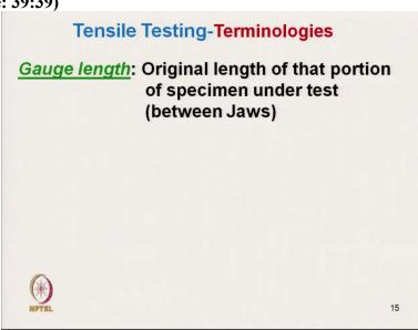
What is gauge length? Gauge length is another term it is the length between jaws ok original length of that portion of specimen under test.
