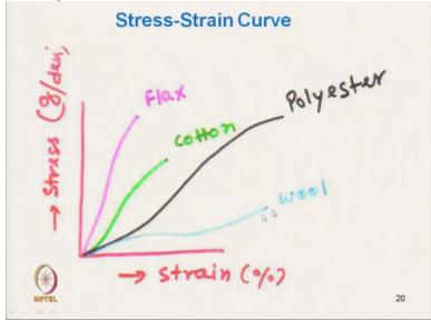
See, wool, polyester, cotton, flax so it changes depending on the molecular structure. Flax has got very high modulus ok due to structural orientation of molecule. So, we will stop here and continue in the next class.
