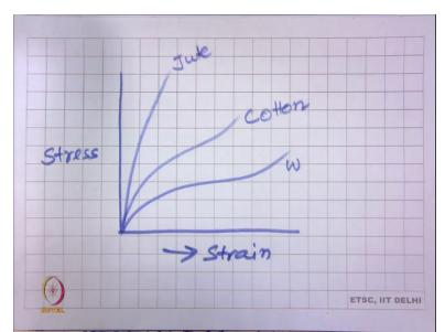
Now let us see, so, this is; these are the three fibres natural fibres this is for wool, this is for cotton, this is for jute. So this difference in nature it is basically due to the molecular structure so, depending on molecular structure nature of curve changes. (Refer Slide Time: 54:18)
