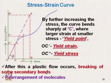
Because within this hook OA zone breakage of bond. Now once it crosses what will happen? By further increasing the stress the curve bends sharply at C suddenly it bends where large strain occurring with small increase in stress. So, that it gains towards the x axis. So, the large strain is occurring with small increase in stress. This particular point is known as yield point and OC dash is yield strain and OC double dash is yield stress.
