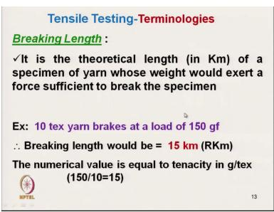
So, now let us see 10 tex yarn breaks at load of 150 gf. That is the condition here one tex yarn breaking at 150 gf what will be the breaking length in kilometre? Breaking length, so, let us see breaking length would be 15km because we can see here10 tex means 10g ok 10 gram of yarn length will be 1km. 1km yarn length 10gm ok that means 15gm, 150gm is the gramforce will have 15km length. 15 km yarn will weigh 150 gf.
