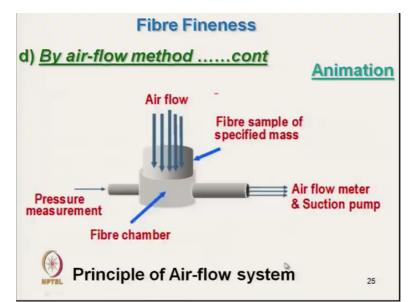
Now the principle here is that the specimen is actually packed here, in the fibre chamber. In the fibre chamber, the specimen is packed. Now with the air suction arrangement, the air is sucked ok, now, air flow with a pump, using a pump, air is actually, sucked. And then the air is flowing and creating certain air pressure, so for certain air pressure. This air flow rate, we can measure.
