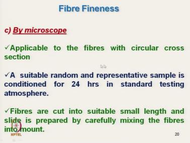
So, where it is a basically we have mentioned that, it is applicable for only circular fibre, where the cross section is circular in nature, and after proper conditioning, we have to put the fibre, we have to mix the fibre into the mount ok. And then we have to mix properly, carefully it is mixed. (Refer Slide Time: 01:02)
