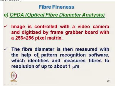
Next is that the image is controlled with a video camera, it is captured with a video camera and digitized by frame grabber so that image processing we can get, ok. The fibre diameter is then measured with the help of pattern recognition software, so that we can measure ok. Light scattering method, this is the, it is called Fibre Diameter Analyzer ok. Analyzer it works in a light scattering principle.
