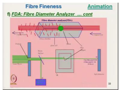
Now this is the arrangement here. See this is the light beam of 200, now here it is a, this is the fibre here, ok. The sensor here, this one is the sensor. And this is splitter, this is splitter, light is splitted in 2 equal part. So here we know the actual intensity of the fibre, actual intensity of the light here. And the fibres are moving. This is with the slurry ok with the liquid flow, with the slurry, with the fibre. It is snippet. It is moving in this direction.
