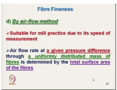
Next method is that, by air flow method. Air flow method, here we measure the fibre fineness, indirectly. It is total indirect method, and here, we do not measure the fibre fineness of individual fibre, it is the overall fibre fineness. Here we cannot measure the, the dispersion, that is the variation of fibre fineness within the, within the particular mass, ok. So what we get, we get a overall fibre fineness, of mass, ok.
