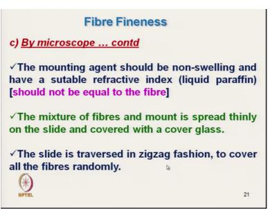
And mount, it is selected in such a fashion, that it should not, should not swell the fibre, and refractive index of the mounting agent should be different from the fibre and typically liquid paraffin is used. And the mixture of fibre and mount is spread properly, on the slide, and covered with the cover glass. And slide is moved in zigzag fashion so that to cover most of the fibres random.
