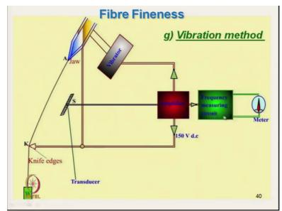
Now this is the technique, here this is, actually the vibrator is there. And here it is vibrated with the wide range of vibration, and where the maximum frequency is there, that value is taken.
