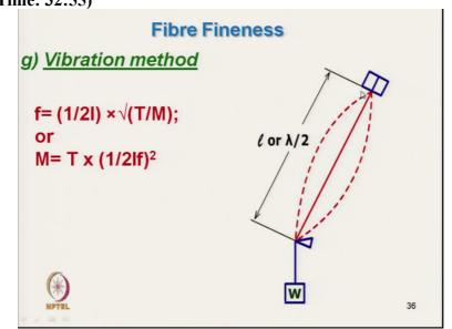
Now this is the, this we know, so frequency that is the natural frequency, is equal to 1/21, multiplied by under root T/M, ok, where T is the tension on the string, f is the frequency, l is the length of the, free length, here, between the 2 point, and M is the mass per unit length ok. In this way using this formula, we can measure the mass per unit length. **(Refer Slide Time: 33:43)**
