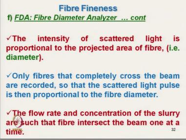
Now let us see, the intensity of scattered light is proportional to the projected area of fibre. So that means the fibre, that is, diameter, more diameter, higher the diameter, higher will be the intensity of light, scattered. So 200 mm, the most of the, all the fibres are less than, what we are measuring is less than, the 200 mm diameter, but what we are measuring, the scattering of light, the scattered light quantity, quantity of scattered light.
