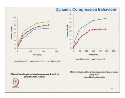
Here the dynamic compression behaviour it shows these are the fabrics. The blue one is made of these are all these are the knitted fabrics. In x axis, it is showing the time of test
