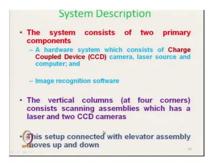
The technique is that here the system consists of two primary components. One is that that hardware component which consists of CCD camera and a laser source and a computer, and second one is that Image Recognition Software. So, these two systems are there.
