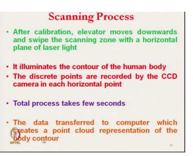
This is the system. After calibration elevator moves downward and swipe the scanning zone with the horizontal plane of laser light, laser light will move horizontal. It will create complete contour. It eliminates the contour of the human body, the discrete points are recorded by CCD camera in a horizontal point, total process takes few second, it moves and the data transferred to the computer which creates a point cloud representation of the body contour.
