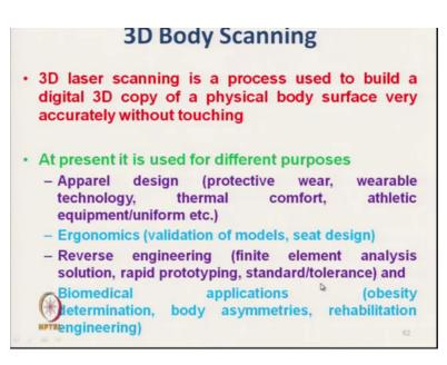
So, latest technique is that 3D body scanning technique and with the 3D body scanning technique here, 3D laser scanning is a process using used to build a digital 3D copy of the body physically digital. It will create a body structure without touching by the use of the laser scanning technique. So, at present this technique is used for different purposes,
