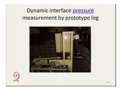
Now, this is the instrument which measures the dynamic characteristics of pressure and quick and wrap our bandage here and this leg, manniquin leg can move at different speed, and as it stretch it is as it bend the knee, there will be a stretching and it will exert the garment will exert pressure. Here the bandage will exert pressure. In our case, we have to use the compression athletic wear,.
