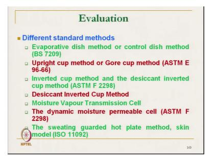
So, different standard methods are available. So, first method is Evaporative dish method or control dish method, which follows the British standards BS 7209 which is evaporative dish method. Similar to that another method is developed by ASTM: ASTM E 96-66; so upright cup method or Gore cup method, Gore cup method or Upright cup method. This is actually it is a evaporative dish method and this upright cup method these are approximately these are same methods. So, we will discuss similar.
