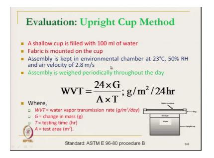
And, calculation is exactly same way we calculate. Here actually we keep the constant water. Earlier we can keep any quantity of water, here the constant quantity of 100 ml water is kept. Fabric is mounted on the cup and it is the temperature and humidity and air velocity is specified and its going and the same way it measures. G is the mass of moisture vapor transmitted, A is the area. So, this way we can measure the moisture vapor permeability by upright cup method.
