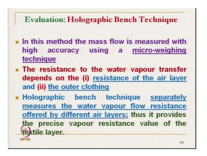
In this method the mass flow is measured with the high accuracy using a micro weighing technique, holographic bench technique. The resistance to the water vapour transmission depends on the resistance of air layer and outer air layer and the outer clothing. So, that
