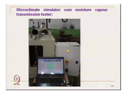
This is the actual instrument ok, this is the air channel and inside the water tank can microclimate portion is there. And, here also we can change the thickness of microclimate depending on our requirement, depending on the; we can change the thickness of this; this can be shifted.
