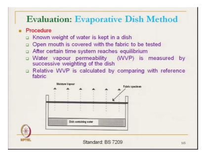
First is that evaporative dish method. In this method known weight of water is kept in the dish. So, known weight of water is kept here and it is kept in a standard atmospheric temperature. Open mouth is covered by fabric ok. After certain time the system reached the equilibrium [FL]; that means, the water flow rate is actually at it at constant rate its water is flowing. So, when it reaches equilibrium the water vapour permeability is measured by successive weighing of the dish.
