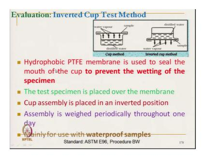
The first the fabric the cup is there and then the mouth is sealed by the hydrophobic PTFE membrane. So, the idea of PTFE membrane it is a porous microporous is there it is a waterproof, but breathable. It does not allow the water in liquid form, but it allows the
