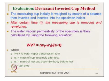
And the measuring cup initially is weighed by the by means of balance and then inverted and inserted into the specimen holder. After certain time the measuring cup is removed and reweighed again. So, the difference is in this way difference is calculated: w 2 is the weight after test w 1 weight before test. So, this is the method. So, this way we can calculate the water vapour permeability.
