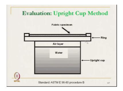
Next is the upright cup method, the system is exactly same only it follows the ASTM principle. Earlier one it follows the BS standard, the same principle air the water is there air layer and the fabric specimen is there.
