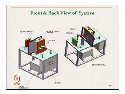
This is typical view of the instrument; here this is the source of heat. So, this is the radiative heat source and along with the burner to give the flame, this is fabric holder fabric sample is there. And this one is the chamber, the climatic chamber where we can control the humidity.
