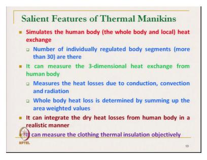
It is basically it simulates the total human body and it is divided into many segments, typically 20 to 30 different segments it is divided and different sensors are placed.
