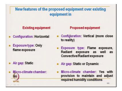
Now, that existing earlier instrument is that it is a horizontal orientation the other most of the other instrument like sweating guarded, hot plate, Tog meter. So, all this instruments are horizontal orientation, but the thermal mannikin is the vertical and it is a 3 dimensional, but this instrument it is a only vertical orientation which is more realistic. The exposure type earlier we have seen in the video it is only flame type exposure, but
