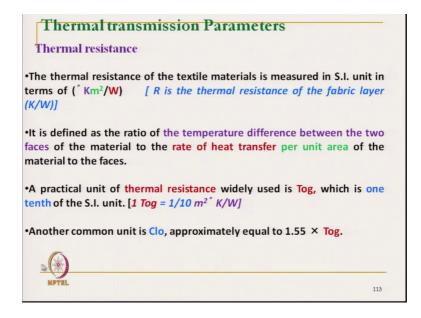
So, what is thermal resistance that we know?Thermal resistance of textile material is a measure in S.I. unit in terms of degree Kelvin square meter by Watt. It is a basically it is a reciprocal of thermal transmittance and which we measured in said sweating I had guarded hot plate we have seen there we measured watt per square meter per degree Kelvin. Here it is just reciprocal of that and R is the thermal resistance of fabric layer.
