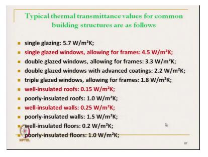
So, we can see the typical values; typical values of some known material, because it is a single glazing type glass so it is a 5.7 watt per square meter per Kelvin. So, these are the different; so well insulated wall it is a 0.25 watt per square meter per Kelvin.
