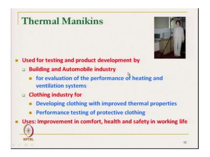
Then coming to another method of measurement of thermal transmission characteristics it is using the Thermal Manikin. Thermal Manikin it gives the idea of total thermal transmission of clothing it is not in the fabric form it gives in the clothing form and it measures the 3 dimensional measurement technique, 3 dimensional it a heat flows at different direction at different dimensions.
