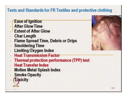
And the type of measurement for fire retardant textile or protective clothing there are different types of parameters one can measure, like ease of ignition. What is that mean say the way that how quick it get ignited, so that depending on the type of fiber, type of finished material, if we can actually use different types of finishing treatment to change this parameter.
