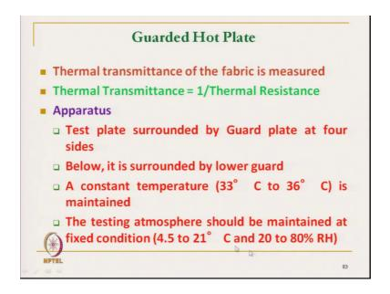
Guarded Hot Plate, here we use the technique of directly the Thermal Transmission measurement by controlling the heat flow from other directions. And thermal transmission is a reciprocal of thermal resistance. And also we have discussed that the test plate is the main component of this instrument which is covered by the guarded plate.
