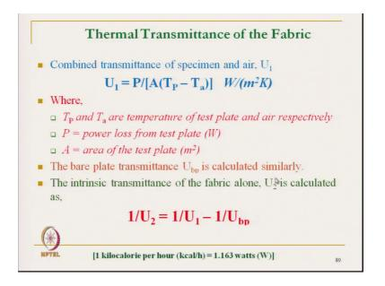
And, now what we have got. So, combined thermal transmittance is what we get, it is a combined means it is a including the layer. So, it is U 1 is the combined insulation; P is the power loss from the test plate, which that means, the power drawn amount of quantity of power drawn by the test plate. A is the area of the test plate and T a T p and T a are the temperature of test plate and ambient air.
