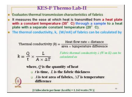
Now, another method measurement of thermal transmission characteristics is the KES-F Thermo Lab ok. It evaluates the thermal transmittance characteristics of fabric where 2 plates are used and in between the 2 plates fabric sample is used.
