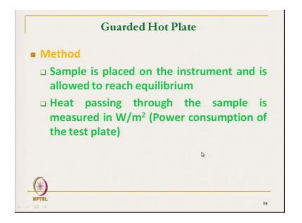
So, the method is that it is sample is placed on the instrument that is the test plate and the temperature is allowed to reach it is equilibrium. And heat passing through the sample, the specimen is measured in watt per square meter, that is a power consumption by the test plate. And as we know that we have to direct the heat flow through the fabric only; heat whatever power is consumed by the test plate that heat has to pass through the fabric only, for that the arrangement is made.
