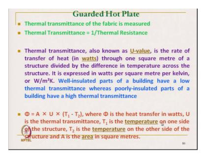
So, thermal transmission is measured here which is a reciprocal of thermal resistance. Now, how do you measure? So, thermal transmittance so, this is the thermal transmittance is also known as U- value. In general it is not only used in textile material it with this U- value it is used for any other place any other place where thermal transmission is important like building.
