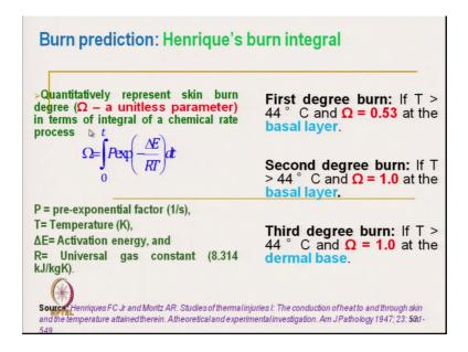
So, these are the 1 ttt a representation of the skin that the omega is the quantitative value. And with this value this is the integral, this value this is the term integral of this omega value it if it is 0.53 it is a first degree burn ok. And if it is 1 that is second degree burn in if it is express in the basal layer and if it is dermal layer then it is third degree burn. So, that way one can get it is a thermal integral. (Refer Slide Time: 33:08)
