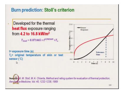
And this is the actually this is the Stoll's curve here. And this is the curve which we have actually got from the instrument this black one and the point where it is actually intersect with this standard curve that is the tolerance time. So, that time if it goes beyond that; that means, then yours third degree burn injuries will start.
