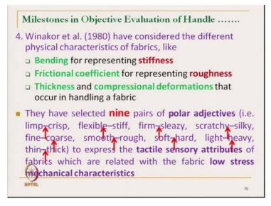
Then Winakor et al in 1980s after that Japanese, they have proposed. They have come up with the wide range of characteristics, wide range of feel. So, and they have correlated with the fabric characteristic like bending. If we measure the bending rigidity, it will give idea about the stiffness of fabric. Whether the fabric is stiff or limp, we can get idea about by measuring the bending rigidity of the fabric.
