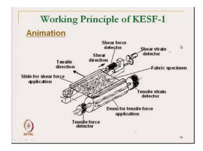
The picture gives the working principle of this instrument. Here this is the fabric sample fabric specimen, which is actually there are two jaws. This is one jaw, which is attached with the rotating drum. This drum when it rotates clockwise, it extends, this gives extension to the fabric sample and gives the tensile load. And during recovery, it gives the recovery.
