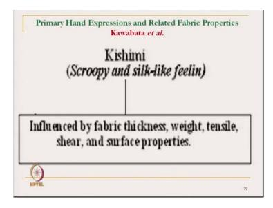
Next one is Kishimi. it is a scroopy or silk-like feeling. So, it is related with the fabric thickness, weight, tensile, shear. So, both tensile characteristics, shear characteristics, and surface property. So, this will give us the value. So, if we keep everything constant, so a tensile characteristics, like tensile elongation or shear characteristics change.
