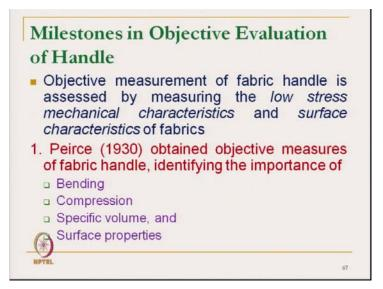
It is actually proposed long back by Peirce in 1930s. And Peirce identified the fabric tactile responses, various tactile characteristics of fabric, which directly sends tactile responses. These are bending, compression, specific volume, and surface property. So, Peirce in 1930s long back, he proposed that if we measure bending stiffness, if we measure compressional characteristics or specific volume of fabric or surface characteristics that these things will give our tactile responses.
