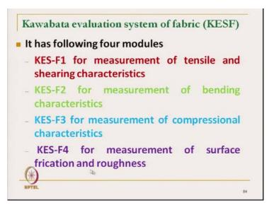
So, KESF they have actually, it is four modules of measuring the low stress mechanical characteristics. So, Kawabata evaluation system for fabric (KES-F1) which actually takes care of the tensile low stress measurement of tensile, and shear characteristics. KES-F2 it measures the bending related characteristics. Fabric bending related characteristics.
