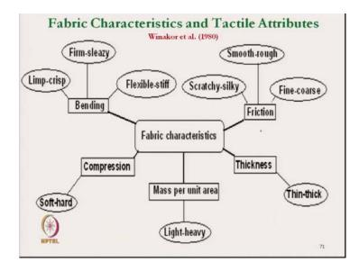
Let us see, how they are related with the mechanical characteristics. Now, try to see limp or crisp, firm or sleazy, flexible or stiff, these attributes tactile attributes are directly related with the bending rigidity. If we can measure the bending of fabric, that they have fabric characteristics that if we can measure the fabric bending characteristics, we can get idea about this polar attributes.
