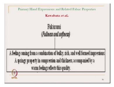
Fukurami, it is a fullness and softness does not mean that it is a fabric, which is soft will give higher Fukurami value. It is a feeling, it is a tactile sensation. A sensation coming from a combination of bulk, rich, and well formed impressions that means, it has to be a bulk and rich value and well-formed impression. And springy property in compression and thickness accompanied by warm feeling that actually reflects this quality.
