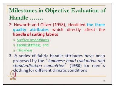
Then in 1958, Howorth and Oliver identified three attributes for suiting fabric. These are surface smoothness, fabric stiffness, and thickness. These are all measurable. So, objectively if we can measure these characteristics, we will get the tactile response. Actually, we can guess the tactile responses of fabrics.
