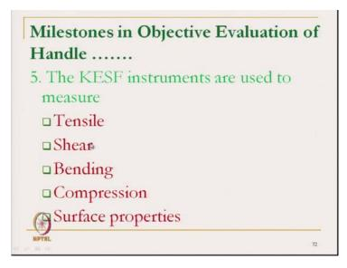
Next measurement is objective measurement is the Kawabata instrument, which is most popular, very popular instrument of objectively measuring the fabric handle characteristics. So, Kawabata system, it measures the tensile characteristics, low stress mechanical characteristics. It is not up to end point, up to the breaking point; it is at low stress mechanical characteristics.
