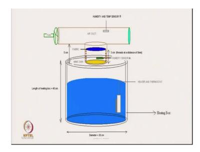
So, we can see there is an instrument, it was developed here to see the microclimate temperature and humidity at different level of air velocity. So, here this is the chamber which actually it is partially filled with water and heater is there to maintain the heat temperature, this is thermostat control; that means, the heater will generate actually that humidity.
