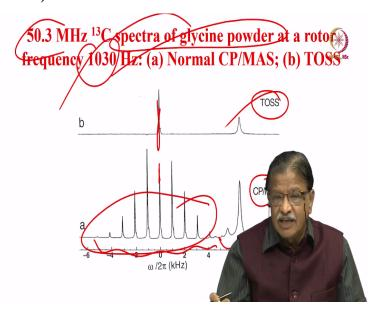
This is simple experiment to show 50.3 megahertz carbon 13 spectrum of glycine powder at this rotor spinning frequency of 1 kilohertz approximately. And this is a normal CP mass spectrum of glycine. Look at it this is for the CO carbon, this is CH3 carbon. Look at this one, how many sidebands are here, lot of sidebands are there. Now, if you do only one
