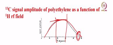
CP time,750 µs, proton rf field was fixed at 5.5 G. MAS speed 2.5 kHz.
