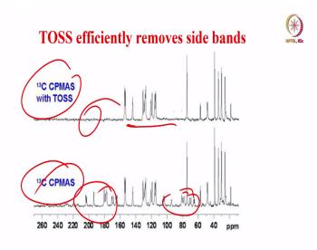
This is the TOSS comparison of glycine powder. It can efficiently remove sidebands in a very complex spectrum like this. Look at this complex molecule carbon 13 CPMA. This is with TOSS, and this is without TOSS. See without TOSS so many sidebands are there. Here now with TOSS all the sidebands are removed; no sidebands. This is an advantage.
