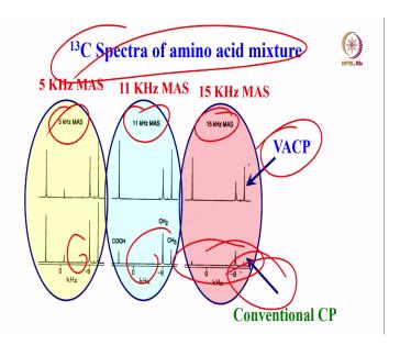
Look at this one. This is what happens if I take the 13 spectrum of different amino acid mixture. Here this is at 15 kilohertz, 11 kilohertz and 5 kilohertz spinning. And here you see the intensity, it is very difficult to match the intensity. Ok, 5 kilohertz is little better. But look at this one,15 kilohertz here, it is very bad now. This is the speed, the intensity of the peaks here. This is because here in these experiments VACP has been done.
