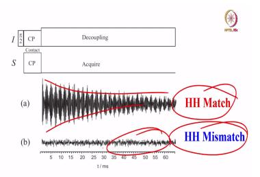
This is the way you adjust the Hartmann Hahn. This is a Hartmann Hahn mismatch condition, the Hartmann Hahn match condition, look beautiful FID you are seeing, when your Hartmann is mismatched, there is no signal at all. This is a normal conventional decouple CP sequence which I said.
