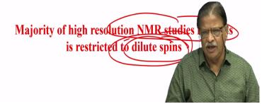
What does it mean? Most of the times, although we say we can get high resolution in protons. As I said it is no way near the comparison with solution state NMR spectrum. Even now the line width is of the order of 40 to 50 hertz, in spite of all technological developments. Lot of stalwarts have devised number of experiments to reduce the line width; varieties of decoupling sequences they have introduced.
