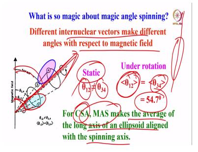
And then what is so magic about the magic angle. Okay I have put the sample in a rotor. Rotor is aligned at an angle with respect to magnetic field and starts spinning at some rapid speed. Some speed 20, 30 kilohertz whatever the speed, I can achieve in a particular rotor. Then what is going to happen? look at it. If you look at it different internuclear vectors are there, which can make different angles with respect to magnetic field, before spinning the sample, you understand.
