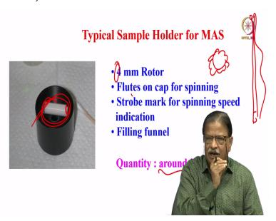
Just to show you a typical sample holder for magic angle spinning, this is like this. It is a rotor and if we take NMR for the solution state it will be like this, a 5 millimeter tube of length about nearly 10 to 12 centimeters and inner diameter about 5 millimeter or sometimes 3 millimeter also are there. But in the case of solid state, since we have to rotate this sample at a rapid speed, the sample is taken in a container like this called rotors.
