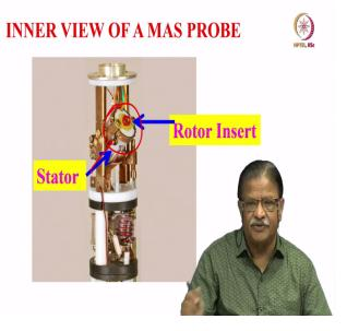
This is a inner view of a magic angle spinning probe. It is different from the conventional liquid state probe. This is where rotor is going to sit, this is called a stator and the rotor goes and sits inside this. There is a small diameter appropriate to the size of the rotor, you have appropriate probe. This is let us say about 2.5 mm rotor, it goes and sits into this, this is the inner view of it.
