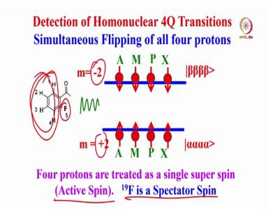
Simultaneously flip all these four protons from alpha alpha alpha alpha to beta beta beta beta and vice versa, all of them from +2 to -2 and vice versa. Then all the four protons are treated as a single super spin called an active spin; 19F is a spectator spin. So, fourth quantum gives you a single peak, because all four protons are simultaneously flipping. But remember fluorine is also a spin half nucleus and the passive spin. It has spin states, alpha and beta.
