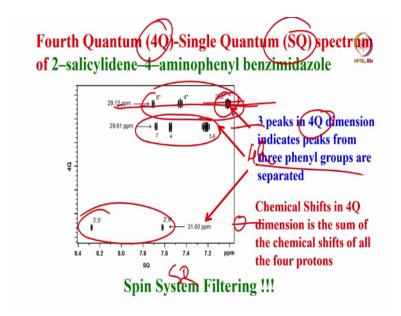
So that is what you can do. So, the 4th quantum single quantum correlation experiment if you do, using the pulse sequence which I showed earlier, in the previous class, which is a homonucler multiple quantum coherence spectrum. Then you are going to get three cross sections here; in the 4th quantum dimension. This is the 4Q dimension. This is SQ dimension, this is called 4Q-SQ correlation spectrum.
