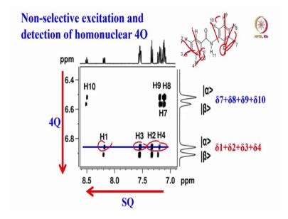
If you take a cross section along this you will get a one dimensional spectrum. Where chemical shift individual protons, in addition to that, the proton proton couplings can be studied here. Hope you understood. You can get proton proton chemical shifts, if you take the cross section of any of these things.
