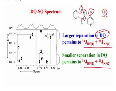
So, this is exactly an example for this in the double quantum dimension. If you do double quantum of nitrogen proton, these two are passive spins, and you can measure the separations and get HF couplings, NF couplings everything, including the relative signs of the couplings based on the displacement vectors.
