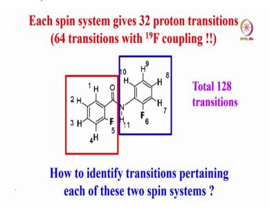
For example, a molecule like this, each phenyl ring gives rise to 32 transitions, each proton, each spin, gives rise to 32 transitions. Here is one spin system of four protons, I am talking about only four protons. Right now, I am not talking about this fluorine and then this fluorine, this phenyl ring gives rise to 32 peaks. This gives rise to 32 peaks. But if it couples with fluorine, 32 will become 64, due to fluorine coupling, will be seen in the proton spectrum.
