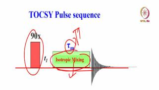
Similar to COSY sequence; instead of second hard 90 pulse, spin lock (isotropic mixing) is used
