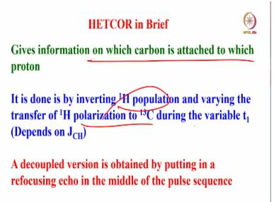
In brief, it gives information on which carbon is attached to which proton; you can also do by it is done by inverting the proton population and transfer of proton polarization to carbon 13 during t1. That is what happens in the t1 period. Although we didnt discuss in stretch. So, you can have the decoupled version, several variants are there.
