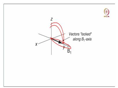
So, what is happening in this case is bring the magnetization from z axis to y axis by a 90 degree pulse. Immediately you can apply a pulse along the y axis, RF pulse, the B1 field now is along y axis where main magnetization is also there. Then what happens is the vector gets locked along the B1 axis, it is called spin locking. The spins are locked along the B1 axis; that is what happens.
