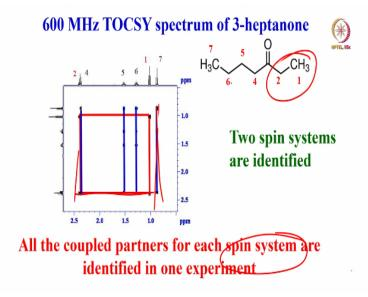
So, now, we will look at the 670 megahertz TOCSY spectrum of simple molecule 3 heptanone. And this is what it is. Now it is going identify the coupled partners in one experiment. What you have to do in COSY you have to go step by step; one is coupled to 2, 2 is coupled to 3, like this you have to keep going, like a ladder. Here, you do not have to do that, in one experiment the entire spin system is identified.
