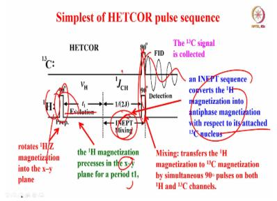
In a simplest form HECTOR looks like this, very simple experiment. A 90 degree pulse before that, there is a preparation period here, everything is done. It is in thermal equilibrium, 90 degree pulse rotates magnetization to the xy plane, here they start evolving; it evolves and precess in the xy plane for a period t1. Evolves under the influence of the chemical shifts of protons and also J coupling between carbon and proton.
