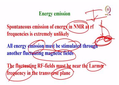
So, now we will talk about the energy emission; How does the energy emission takes place and everything. Of course, as we already discussed with energy levels, the spins in the upper energy state comes to the lower energy state simultaneously lattice ow from lower energy state to higher state, that is what we discussed. There is no doubt about it.
