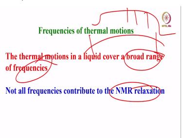
Then what is that which is required? what are the thermal motions that are required? The frequencies of the thermal motions should be of the order of Larmor frequency. Larmor frequency at which the spins resonate. The interaction frequency, the energy of interaction should be of that order, it should be thermal motional frequency should cover the broad range of frequencies so that it will contribute to NMR spins relaxations.
