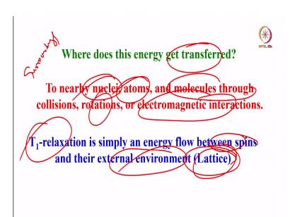
Now you may ask me a question, okay, the system is losing energy, fine I understand. But where does this energy gets transferred, where does it go, how does the system absorbs this energy which is lost by the spin system. This energy has to be transferred somewhere; and it gives its energy to other system. It could be nearby nuclei, it would be nearby atoms and also molecules through collisions, rotations or electromagnetic interactions, varieties of interactions can be there.
