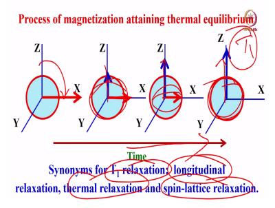
Pictorially in the vector diagram I showed like this. Immediately after the 90 degree pulse magnetization is brought to X or Y axis by 90 degree pulse. Immediately then there is a statistical phase coherence; all the spin vectors are aligned along this axis, but with time what happens the spin start dephasing in the XY plane; I will come to that later, that is called another type of relaxation.
