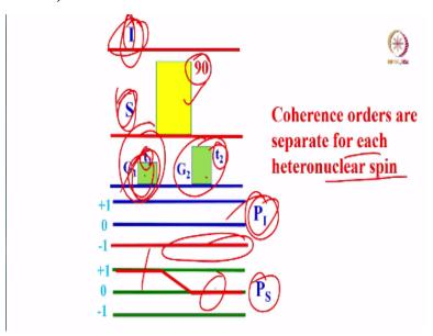
Now I am going to put a diagram like this, this is I spin; notice, I have not applied any pulse on I spin, No need to apply pulse on I spin, but they are coupled; coupling is there. And this is S spin, on the S spin I apply 90 degree pulse. The gradient before the pulse is G1 duration is t1, gradient after the pulse is G2 for the duration t2. Please understand, pulse is not applied only on I spin, but the gradient is applied on both, gradient is general, it is not on a particular spin.
