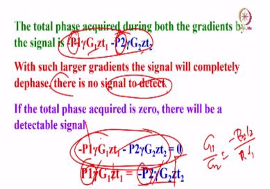
We saw that if it is nonzero then what happens is complete signal will be decaying; the phase acquired is P1 into gamma into G1 z into t for P1 and then for it is P2 is similar; both are negative. If you take the sum, if it is nonzero, there is a complete dephasing.
