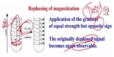
This is only true provided the spins stay in the same slice and don't change their position along the z-axis in the time between the two gradient pulses (No translational diffusion)
