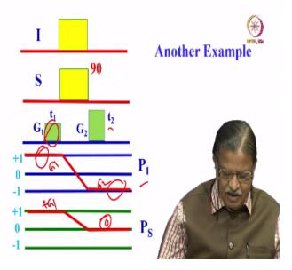
And this is simple example we have chosen. Let us take another simple example now, another simple example is this one; for PI it is +1 during t1 and it is -1 during t2; that is +1 during gradient 1, -1 during gradient 2. This is for gradient 1 this is for gradient 2. What about PS? what is the pathway for S? During the gradient 1, this is +1, during gradient G2 this is 0. Now,
