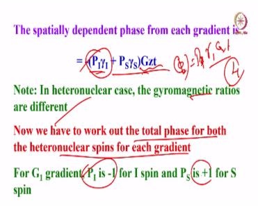
This all the logic I we have to understand. Now, we calculate the spatially dependent phase for each of these gradients. We know how to calculate the phase; that is already given. earlier gammas are same, the gammas are different now, now PI gamma is multiplication factor, this is Gz into t. So, earlier you did P1 gamma Gzt; we wrote. This is phi z; this was the phase acquired for a particular coherent order that we knew.
