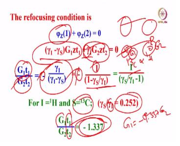
What is the refocusing condition, sum of both the phases should be 0, in which case you can get the detectable signal. So, phi z1 + phi z2 should be equal to 0. Put this condition now, you worked out for phi z1 it is gamma I gamma S into G1 zt1 + gamma I G2 zt2 this is equal to 0. Do this simple jugglery by rearranging the terms. Now, G1 t1 / G2 t2 turns out to be gamma I divided by this term, because both are positive here, this negative sign is carried forward.
