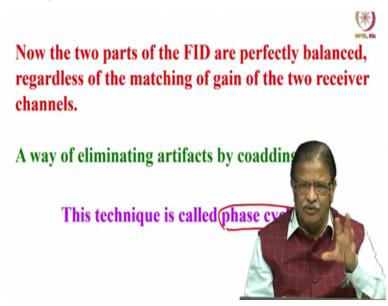
2 parts of the FID, the real part and imaginary part are perfectly balanced, does not matter whether the 2 receivers were matching or not, the gain may be different, but as far as we are concerned, when we start collecting the signal we have managed in such a way that both real part of the signal and imaginary part of the signal get completely balanced.
