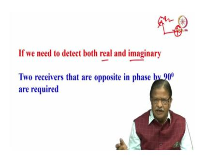
So, now, you may ask me a question I need to detect both the signals. How do we do that? Of course, in NMR that is what is done, we detect both the real and imaginary part of the signal. That means we have 2 receivers that are kept out of phases by 90 degree; this is called quadrature detection. I told you in earlier course, what is the quadratic quadrature detection.
