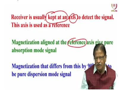
For example, receiver is usually kept at an axis to detect the signal; of course this should be possible even with the first class we told you, a magnetization is along Z axis, you apply a pulse on the X axis, you will have a receiver along Y axis to detect. So, they are all orthogonal to each other; all the three. The directions of application of the pulse, thermal equilibrium magnetization, and the detection, the receiver you are going to keep, all the 3 orthogonal to each other.
