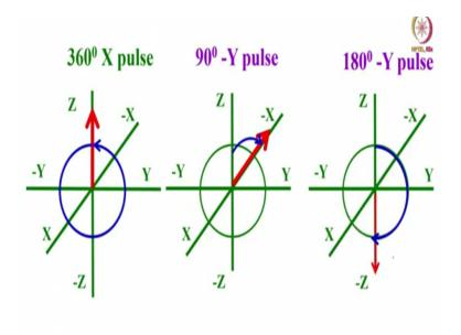
So, this is what happens, this is a clockwise rotation. So, we keep rotating from here, if you see from the center of this, you can see the rotation of the magnetization. So, now, we can also apply the same thing apply 90 degree -Y pulse instead of along plus axis, you apply along -Y axis. See what happens? the magnetization rotates in the opposite direction, you take it -Y, -X axis and then continue further; 180 will take it to, -Z.
