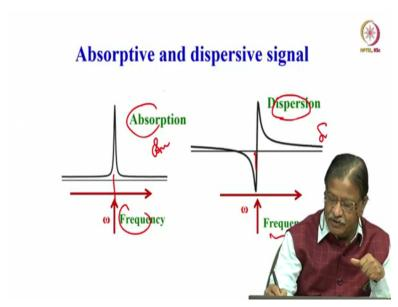
So, what is the absorption mode signal, what is dispersing mode signal? This is the absorption mode signal where you can see the signal positive and it is completely absorbed this is center of the peak and it gives the frequency of it. And this is in general called as an absorption mode
