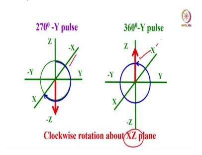
And then further 270 will take it to +X and then 360 again brings it back to Z axis. Again one complete rotation of the magnetization you can do. So, what have we understood so far. You can have the amplitude and power of the pulse; the width and power of the pulse you can tune it in
