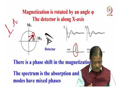
Now allow the magnetization rotate by any angle phi; as I told you it is somewhere here; what is the signal you are going to get? Now, you have a MX component as a MY component both are present here; MX and MY both are present. So, it is a mixture of absorptive and dispersive; see here it is not absorptive, there is a phase error here, phases if it is really pure signal there should not be any phase error; it should be like this, here there is phase error like this signal.
