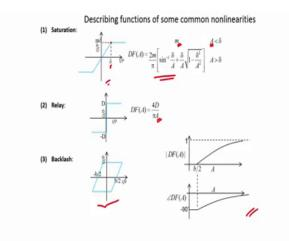
So, we shall first start with the saturation nonlinearity and the input output relationship has been shown here. So, the output is proportional to the input up to some either voltage or value which in this case has been called as delta. And if you write down the describing function, we note that sinusoidal signals of amplitude between 0 and delta, we would have the describing function to be equal to simply the slope of the straight line that relates the input to the output.
