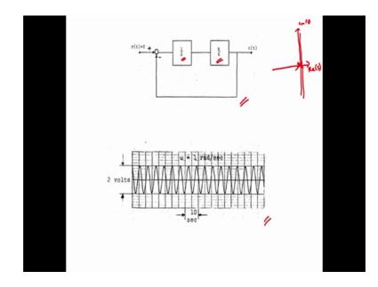
So, what you see in the block diagram at the top is a conventional linear control system with the plant being an integrator namely k by s and the controller also being the an integrator 1 by s. So, we have just 2 integrators as part of our open loop dynamics. Now if 1 were to plot the root locus for a system which has 2 integrators as part of its open loop dynamics, when in other word from plotting the real part of s verses the imaginary part of s, we have 2 open loop poles at the origin.
