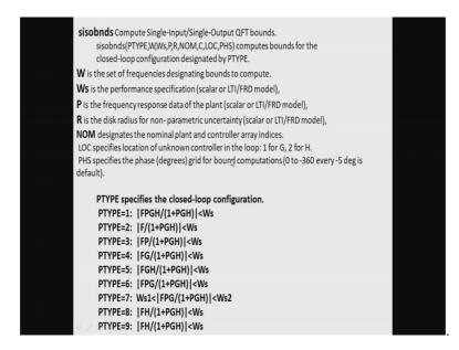
So, in this power point slide I have pasted the result of piping help siso bnds in the MATLAB command window and this is the information that you get regarding this particular function. So, it has several input arguments, it is intended to compute the bounds for problems of different types. So, the first input argument to this function is the problem type or p type.
