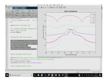
So, what you will see therefore, here are the bounds on the loop gain at different frequencies in order for us to achieve robust tracking, these bounds have been color coded. So, the red bound at the top which I am showing by means of the arrow here corresponds to the bound on the loop gain at 0.2 radians per second and what it essentially implies is that in this Nichols plot the loop gain, the nominal loop gain has to
