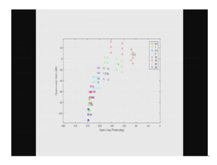
Now, we can repeat this exercise of other frequencies also, in the frequency vector that we have just defined. And the plant templates at the different frequencies are all plotted together in this graph here. So, they have all been color coded for instance, the red circles at the top represent the plant template at 0.2 radians per second.
