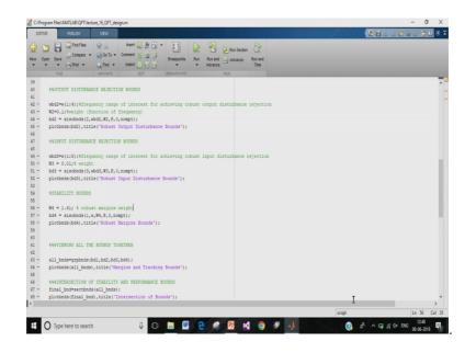
Now, in this particular quote we have to convert db to the linear scale. So, 3 db essentially come gets converted to 1.41 units in the linear scale. So, the performance specification for stability is w 4 and is equal to 1.41 units, which essentially signifies that the maximum value of our feedback part of the transmission function t 1 should be less than or equal to 3 db. So, subsequent to drawing all the bounds we would wish to view all the different bounds that exist for our loop gain.
