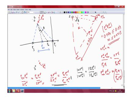
To understand the geometric meaning of this equation, I have written down this expression once again and alongside it above it I have once again the complex plane displaying the locations of the different open loop poles and the desired dominant pole location on the right hand side, I have separately zoomed in to the area near the 0 z and indicated the point z in relation to the point P C L naught.
