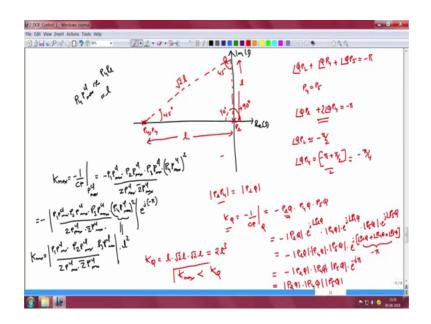
So, in this schematic here I have now replaced the three poles and two zeros which were near the origin with a simple single lumped pole which is how this combination would appear for the point Q which is on the branch of the root locus that is very far away from this combination of poles and zeros.
