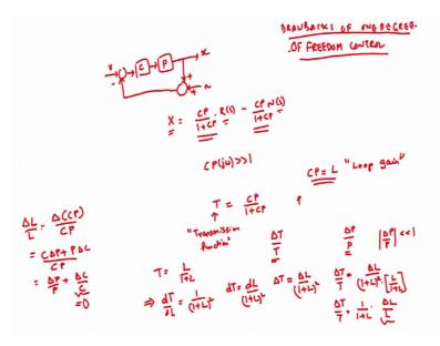
The output of the plant is of course, measured by a certain measurement system and is fed back and compared with the reference R. But invariably when we are making a measurement we cannot avoid some measurement noise n keeping in and affecting the actual measurement.
