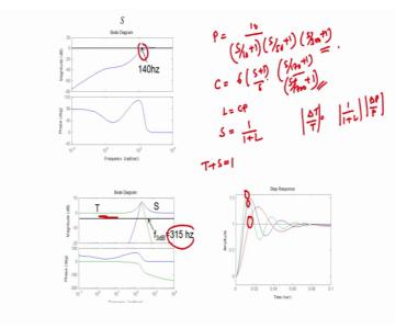
I have in the next slide plotted a sensitivity function for the overall closed loop system that we had, when we when we undertook the design using Bode plots. So, to remind you we had the plant P to be equal to 10 by S by 10 plus 1 times S by 50 plus 1 times S by 300 plus 1 this was the plant transfer function.
