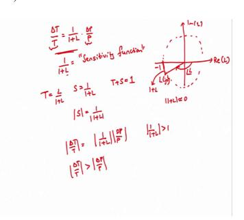
With the consequence therefore that the relationship between the uncertainty in the transmission function delta T by T and the uncertainty in the plant delta P by P is given by delta T by T is equal to 1 by 1 plus L times delta P by P. So, delta P by P represents the fractional uncertainty in the plants model, and delta T by T represents the
