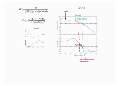
So, the principle states that A signal r of t or a disturbance d of t can be rejected perfectly in steady state, if the denominator polynomial of R of s which is a Laplace transform of R of p or D of s is included as part of the denominator polynomial of the controller C of s. So, if we include the denominator polynomial of r of t of d of t as part of the denominator polynomial of our controller C, then we can in steady state reject the disturbance perfectly, but track that reference perfectly.
