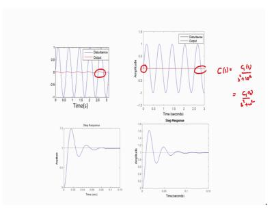
In this case I have carried out a simulation where we have compared the performance of the close loop system in the absence of this controller. So, this is the original PID controller that we had designed a few clips back, and we discussed that you are able to bring down suppress a disturbance by 99 percent, exact 98 percent, exactly as we had desired it to be although it was not completely suppressed.
