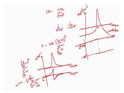
So, what I use to do, is to have a controller C of s to be of the form C 1 of s divided by s square plus 10 square, why did we choose 10, that is because that is the frequency of the disturbance that we want to reject in this particular case
