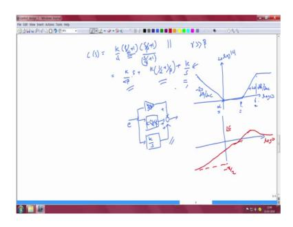
In this in these lectures we have represented PID controllers in this particular form. K by s times s by alpha plus 1 times s by beta plus 1; where this 0 alpha is intended to improve the mid frequency performance and 0 beta is intended to improve the high frequency phase characteristics and thereby result in a stable closed loop system.
