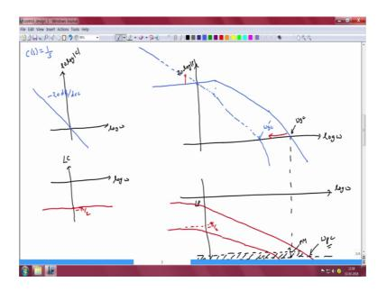
So, the transfer function of an integral controller is c of s is equal to 1 by s. If you want to draw the bode plot of an integrate an integral controller. We would have the magnitude characteristic to be a straight line of slope minus 20 decibels per decade and the phase of this transfer function when we set s is equal to j omega, we will see that the phase angle of c will be equal to minus 90 degrees, so minus pi by 2 at all frequencies.
