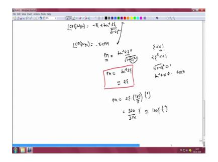
From the previous slide we have angle of CP at the gain crossover frequency to be equal to minus pi plus tan inverse 2 zeta by square root of 1 minus 2 zeta square and by definition of phase margin. We know that the angle of CP at j omega c omega g c is by definition equal to minus pi plus p m, where p m is the phase margin of our open loop system.
