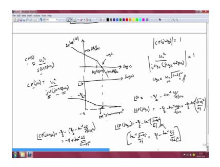
So, to remind you from the previous slide, we have the open loop approximate transfer function this is not the exact transfer function, because we have not yet designed the controller c. In order for us to get the approximate closed loop transfer function that we wrote out in the previous slide, the approximate open loop transfer function look should look something like this omega n square by s times s plus 2 zeta omega n.
