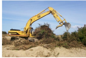
An excavator machine is made up many pieces joined together. The movement at the joints are constrained.
