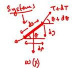
How can we understand this? You can simply think of it this way that: if I have the same amount of dx, the horizontal component, but at a different; consider two pieces of rope, which has the same amount of dx, but one is the angle makes with the horizontal is  $\theta_1$  and the other one is a little bit more bent towards the upward direction. So, this is  $\theta_2$ ,  $\theta_2$  is greater than  $\theta_1$ .
