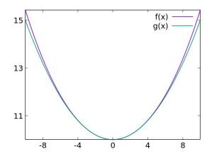
One of these functions is mentioned here, So one function represents this cos hyperbolic function, and the other function represents the parabolic function; these are the functions chosen so that it matches the equation that we found from our analysis, So, this will represent a massive rope or
