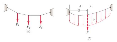
So, in this particular problem, we are going to assume that this is the case. So, now let us define the example more concretely. So, as I mentioned so these are two ends which are fixed and these two ends, A and B, and there is a cable whose length is I which is hanging between two ends. Note that these two ends, in general, can be at different heights. So, they need not be symmetric.
