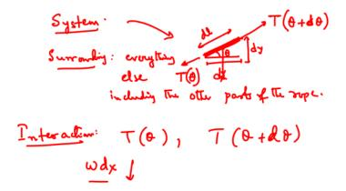
So, it is a small piece of rope, and this makes, this piece makes an angle  $\theta$  with the horizontal if the x axis. Then this is the tension. So, this is my system and everything else is surrounding is my system and everything else is surrounding which includes the other
