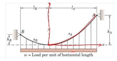
So, I have chosen the lowest point of the row as my origin, and then I have chosen the tangent to the lowest point as my x-axis and the perpendicular direction as my y-axis. So, this is a deliberate choice to make the shape very simple and the equation of the shape as simpler as possible. And as you can expect, in general that if you shift the origin, then the equation of the curve will shift will also change. So, let us try to analyze. So, first thing is what is going to be our system.
