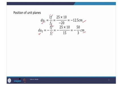
How to get the position of unit plane, we will use the formula which is derived earlier,  $d_{u1}$  which is the position of the first unit plane which is given by  $tf/f_2$ , just substitute for tf and  $f_2$ , you get a position of first unit plane, substitute again for tf and  $f_1$  and this will give you the position of the second unit plane. This is how we can easily calculate the position of unit plane, matrix elements, focal length, very easy.
