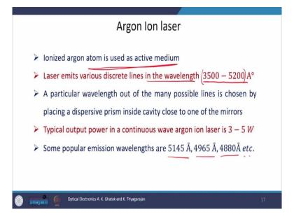
Apart helium neon laser, argon ion laser is another important gas laser. In argon ion laser ionized argon atom is used as an active medium. Now, this laser emits various discrete lines in wavelength reason lying between 3500 to 5200 Angstroms and this wavelength band this laser emits several wavelengths, its emit several discrete lines. A particular wavelength out of many possible line is chosen by placing a dispersive prism inside cavity close to one after mirrors.
