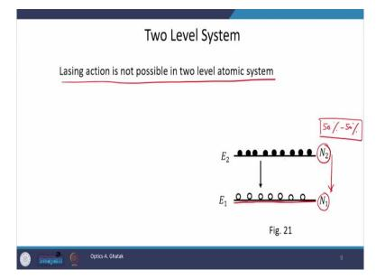
Now, lasing action is not possible in the two level system and we have already understood it because we know that the rate of transition from lower energy state to upper energy state is proportional to  $N_1$  which is the carrier density in the ground state and the rate of transition from upper state to lower a state is proportional to  $N_2$  and in two level system we can at most have 50-50 distribution of carriers or electrons.
