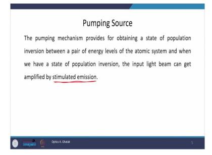
Now, pumping mechanism provides for obtaining a state of population inversion between a pair of energy levels of the atomic system and when we have a state of population inversion, the input light beam can get amplified by stimulated emission. If you remember in the last class we studied about three phenomena, stimulated emission, spontaneous emission and absorption.
