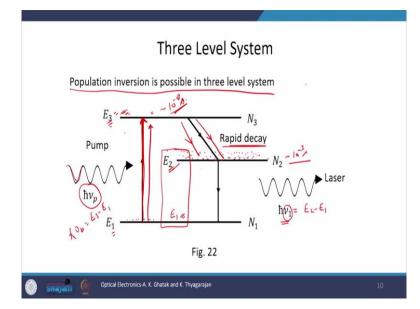
But in three level atomic system we can make a laser, why? because, now, the atoms or electrons from  $E_1$  level is pumped to higher energy state which is  $E_3$  here. The pump has a frequency which is equal to  $E_3 - E_1$ , here  $\hbar v_p = E_3 - E_1$  and in this situation the electron will directly go to the third energy state.
