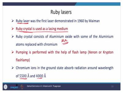
Now, Ruby laser was the first laser demonstrate in 1960 by Maiman. Now, Ruby crystal, as the name suggests, the Ruby crystal is there in this laser. Therefore, Ruby crystal is used as a lasing medium in ruby laser. Now, in this laser, it is not the pure Ruby crystal, because Ruby crystal is made up of aluminium oxide,  $Al_2O_3$ .
