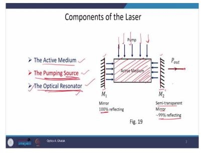
And today, we will formally start with the laser. Now, this slide is dedicated to the component of a laser. The laser consists of three main components, the first one is active medium, active medium consists of ions, atoms and molecules. Now, these atoms, ions and molecules provide the discrete energy levels where in we after achieving population inversion, we get lasers, we get light out of the out of these systems.
