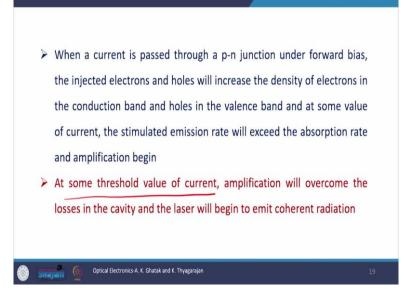
Now, when a current is passed through a p-n junction, under forward bias, the injected electrons and holes will increase the density of electron in the conduction band and holes in the valence band. And at some value of current the stimulated emission rate will exceed the absorption rate and amplification begins.
