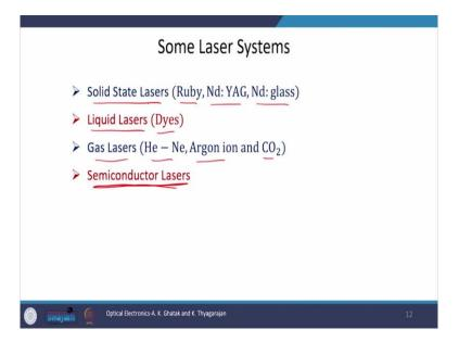
Now, a few examples of laser systems are solid state lasers, liquid lasers, gas laser, semiconductor lasers. Now, in solid state laser, Ruby, Nd: YAG, and Nd: glass are most famous ones. Dyes lasers are examples of liquid lasers. Helium, neon, argon and CO2 lasers are examples of gas lasers. In modern communication system, it is now semiconductors laser which are dominating the field, we will study about these lasers.
