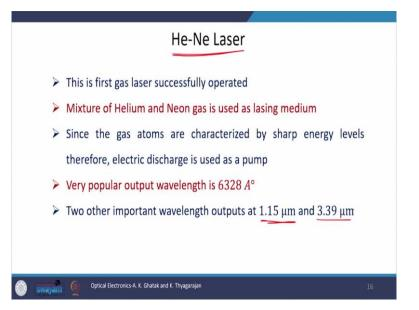
Now, coming to gas laser, the most important and widely used in street laser is helium neon laser. This is the first gas laser which operated successfully in this laser helium neon is the active medium, mixer of helium and neon gas is used as a lasing medium in this laser since the gas atoms are characterized by sharp energy levels.
