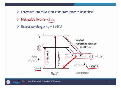
Now, here you can see the energy levels of chromium ion. This is the ground state and you see that it is absorbing 5500 Angstrom and it is going in energy level  $E_1$  while the absorption at wavelength 4000 Angstrom lead the electron to the uppermost energy level which is  $E_2$  level.
