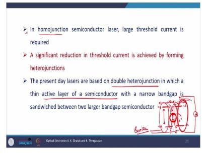
These were the different kinds of laser but, a few more important properties of the semiconductor laser is that, there exists two configurations of the semiconductor laser, one is called homojunction semiconductor laser and another is called heterojunction. In homojunction semiconductor laser, the large threshold current is required while a significant reduction in threshold current is seen in heterojunction semiconductor laser.
