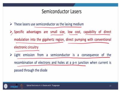
The next important laser is the semiconductor laser. They are widely used in our communication system nowadays as the name suggests, these lasers use semiconductor as the lasing medium since it is a solid state laser. And therefore, they are not bulky of course here and therefore the specific advantages of semiconductor lasers are small size, low cost, capability of direct modulation into gigahertz region. We can directly modulate these lasers at a very high speed gigahertz region.
