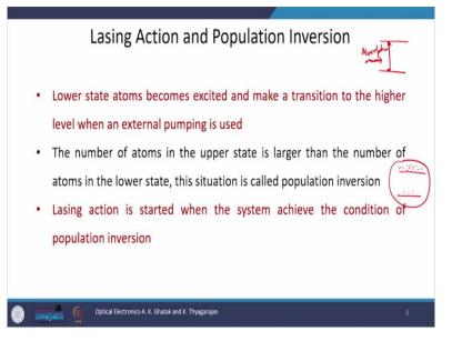
Now to achieve lasing, we require population inversion, lower state atoms becomes excited and make a transition to the higher level when an external pumping is used this we know. If the electron is here, then if you pump it then it goes into the upper energy state. And it only happens when we have some external source and this is called absorption.
