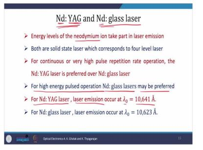
Now, similarly Nd: YAG and Nd: glass lasers are also important, the energy levels of neodymium ion take part in laser emission. Now, both of these laser Nd: YAG and Nd: glass they are solid state laser and they both are 4 level. Now make it a point Nd in both the laser stand for neodymium while YAG stands for Yttrium Aluminum Garnet.
