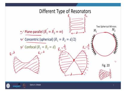
This is the simplest example of a resonator and there are different kinds of resonator, the simplest one is shown here, you see there are two curved mirror facing each other and this
