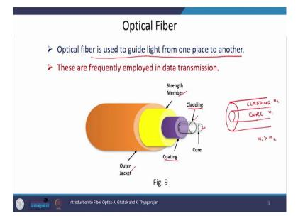
Therefore, the optical fiber is used to guide light from one place to another and these are frequently employed in data transmission. Whatever communication we do long distance of course, long distance communication like we use mobile phone and then the data from our mobile it goes to some antenna and from antenna it get coupled to a waveguide.
