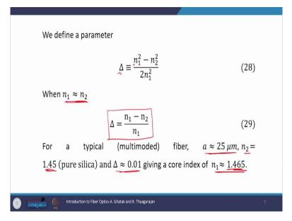
Now, moving ahead, while analyzing an optical fiber, we define a parameter which is called  $\Delta$  which defines relative refractive index difference between core and cladding, which is defined as  $(n_1^2 - n_2^2)/2n_1^2$ . But usually in fiber,  $n_1$  is very close to  $n_2$ , this is done to reduce dispersion which we talk about in coming slides.
