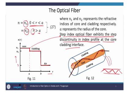
In optical fiber as I said before, the core refractive index is larger than that of the cladding. Therefore, if you launch a light which is larger than critical angle for refractive indices of core and cladding, then it will suffer total internal reflection at core cladding interface and this way it get guided along the length of the fiber.
