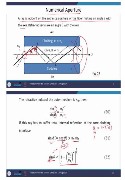
Now, we will define new terminology which is Numerical Aperture. Now, in this figure, figure 13, we present a cross section of an optical fiber where this white region represents core and this shaded region represents cladding. Basically, it is cylindrical, but I am showing you the cross section of this optical fiber.
