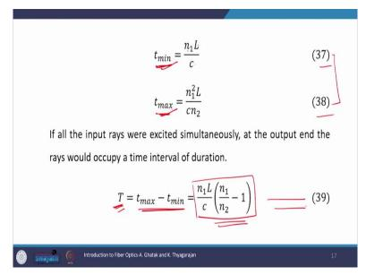
Now, we can quickly write the expression for time minimum and time maximum as  $n_1L/c$  and  $n_1^2L/cn_2$ . Where we use this formula, equation number 36 here. In 36, in first case we replace  $\theta$  by 0, and in the second case we replace  $\theta$  by  $\theta_c$  which is equal to  $cos^{-1}(n_2/n_1)$ . This gave us  $\theta_{min}$  and  $\theta_{max}$ .
