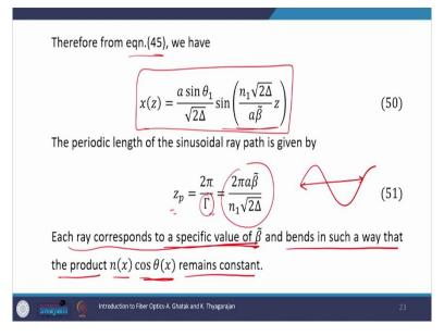
Now substituting the expression of  $\Gamma$  back into equation number 45 get this ray equation. Now you see that it is a sinusoidal function, then therefore we can easily calculate the periodicity which is given by  $2\pi/\Gamma$  and from here, after substituting the value of  $\Gamma$  we get this value of  $z_p$ , the periodic length of the sinusoidal ray this made this means this length.
