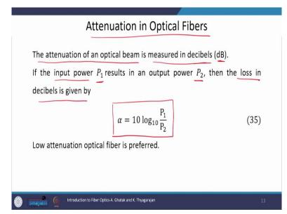
Now, let us talk about attenuation in the optical fiber. We know that optical fibers are made up of silica glass, because we want the light to propagate inside it and it must be transparent otherwise that light would be lost. But irrespective of the transparency of the glass, there are
