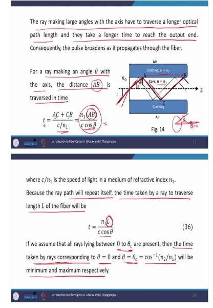
Now, the ray making larger angles with the axis have to travel longer optical path length and they take longer time to reach at the output end, this we already discussed the dash ray it is making larger angle with respect to the optical axis of the fiber while the continuous black line black ray, it is making smaller angle therefore, the dash ray will take longer time to reach the output. And consequently, the pulse broadens as it propagates through the fiber.
