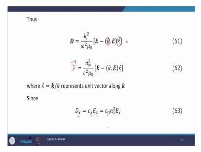
Now, let us simplify it we take k the magnitude of k outside of this bracket then equation number 60 becomes a equation number 61. A further simplification leads to equation number 62 you are seeing  $\hat{k}$ .  $\hat{k} = \vec{k}/|\vec{k}|$  which is unit vector which points along vector k, and we know that  $D_x = \epsilon_x E_x$  which is in principle coordinate system and  $\epsilon_x$  is nothing but  $\epsilon_0 n_x^2$  which we already which we have already seen.
