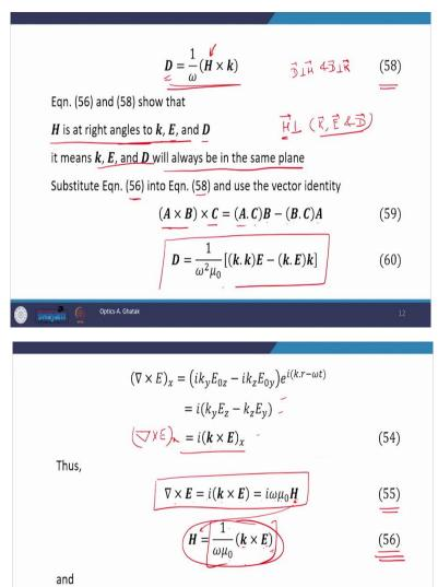
And from here we get the expression for D here D is here on the right-hand side and the expression  $D = 1/\omega(H \times k)$ . It means D is perpendicular to H as well as D is perpendicular to k. This is what equation 58 says. Similarly, this equation says that H is perpendicular to k as well as H is perpendicular to E.
