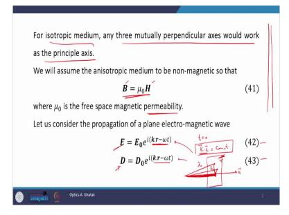
For isotropic medium therefore any three mutually perpendicular axis would work as a principal axis. Now, we will assume the isotropic medium to be nonmagnetic, this would simplify our mathematics therefore,  $\mathbf{B} = \mu_0 \mathbf{H}$ . Where  $\mu_0$  is the free space magnetic permeability you are hearing these two words permittivity and permeability.
