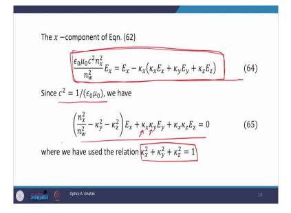
Therefore, the x component of equation number 62 can be written as this. The equation number 62 the x component of equation number 62 is written like this here. Where in what we did is that we pick the x component of D then the x component of E and x component of k,  $\hat{k}$  which is outside the bracket. Now, we already know that  $c^2 = 1/\epsilon_0 \mu_0$  bit of simplification gives equation number 65.
