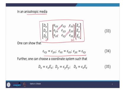
Therefore, in anisotropic medium this relation holds between D and E. Where the matrix on the left-hand side is component matrix of displacement vector D, this matrix is the component
