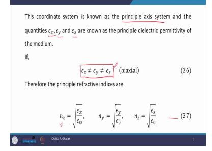
Now, there are two cases, the first case is of biaxial system where in  $\epsilon_x \neq \epsilon_y \neq \epsilon_z$ . Anisotropic material in which this relation holds is called biaxial material or biaxial crystal. And in these
