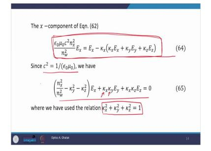
Now, similarly, we can write the y component as well as z component. This is our  $E_x$  component this is y component and this is z component of the same equation. Now, these equations equation number 65, 66 and 67 they are the component of the same equation and there are three homogeneous equations you see on the right-hand side here we have 0.
