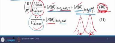
And after a bit of calculation, we can get the expression of  $\Delta\delta$  and which for the large value of F, which is coefficient of fineness would be equal to  $4.2/\sqrt{F}$ , what does this represent? This represents the smallest phase increment,  $\Delta\delta_{min}$  separating the two resolvable fringes.
