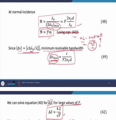
This represents the smallest phase increment,  $(\Delta \delta)_{min}$ , separating two resolvable fringes. From eqn. (28)
