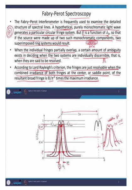
Application of Fabry-Perot interferometer is predominantly in spectroscopy. The Fabry Perot interferometer is frequently used to examine the detailed structure of spectral lines, a hypothetical purely monochromatic light wave, just observed this word hypothetical because it is impossible to have a purely monochromatic light source.
