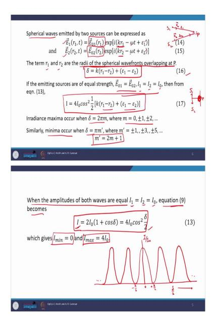
Till now, we were considering that the waves which are arriving at the point of observation P are plane but what will happen if we put the point of observation P close to the sources or alternatively what will happen if the waves reaching at point P, the observation point are spherical not plane.
