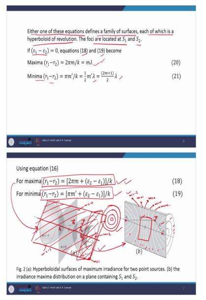
Now, as I discussed earlier either one of these equations, which equations? These equations equation number 18 and equation number 19, they defines a family of surface, each of which is a Hyperbolide of revolution and the foci are located at sources  $S_1$  and  $S_2$ .
