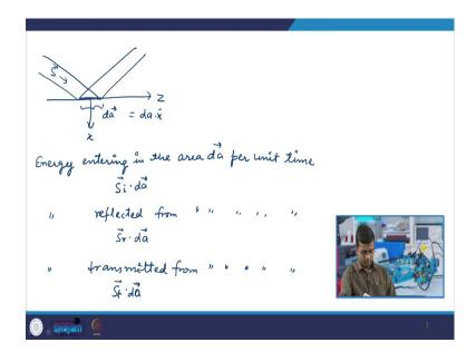
So, this is our interface. A beam is coming like this, it is getting reflected from here and this is the area. So, it was x direction if you remember, this is z direction this is S now flowing in this direction and this is da, the area where it is falling that is da into x. So, energy entering in the area da per unit time - S i dot da. Similarly, energy reflected from area da per unit time is - S r dot da. Energy transmitted from area da per unit time is S t dot da.
