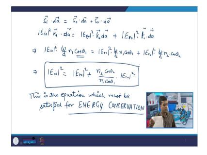
So, in principle, S i dot d a should be equal to S t dot d a plus S r dot da; that is mod E i 0 square k 1, k 1 is equal to into da is equal to mod E r 0 square into k 2, k 2 it is also k 1 no, this one is k 2 dot da r t actually plus mod E r 0 square dot k 1 dot da. k is small actually sometimes I write it seems like capital, but it is small k.
