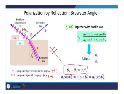
So, what happens? At Brewster angle r p goes equal to 0 and you see that we can have this ray like this. You have electric field components in the plane and electric field components out of the plane. So, these ones - components perpendicular to the page and components parallel to the page. So, this one is parallel to the page - this is called p polarization, and this is called s polarization or TE. And this is TM - Transverse Magnetic.
