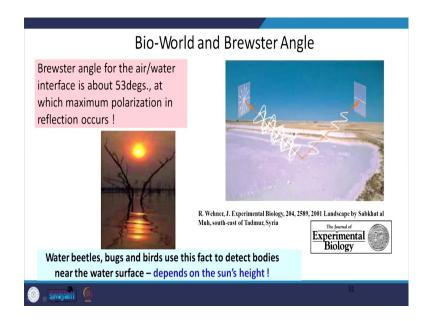
Brewster angle for the air water interface is about 53.5 degrees at which maximum polarization by reflection occurs. So, you can see that when the angle is large, say, during the morning or evening times you have maximum polarization in reflection. So, sometimes you do not see, even, reflection only if you are using a p-polarized light.
