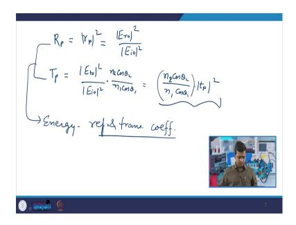
So, from her if you want to calculate what are the R p - is equal to simply mod r p square and that is equal to E r 0 squared divided by E io square and T p - is equal to which is mod E t 0 square divided by E i 0 square into n 2 cos theta 2 divided by n 1 cos theta 1
