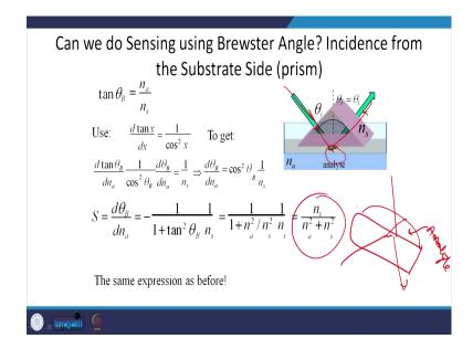
If we want to use it other way around like on a substrate we were putting a drop and we were shining from here. So, here was the analyte, which you do not prefer most of the time. Can we put light from here and see what happens and measure the reflectivity here? That can be attained by using a prism.
