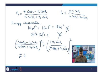
So, let us see the reflection coefficient, that was n 1 cos theta 2 minus n 2 cos theta 1 divided by n 1 cos theta 2 plus n 2 cos theta 1, this was the reflection coefficient. And the transmission coefficient t p was equal to 2 n 1 cos theta 1 divided by n 1 cos theta 2 plus n 2 cos theta 1. So, we had these two.
