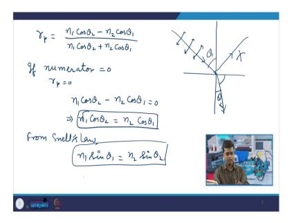
So, we know that r p is equal to n 1 cos theta 2 minus n 2 cos theta 1 divided by n 1 cos theta 2 plus n 2 cos theta 1. If numerator is equal to 0, then r p is equal to 0. What does it mean? It means that, for p-polarized light: p -polarized light means that the electric field component which is in the plane of the incident light will not be transmitted. So, there would not be any reflection for this electric field.
