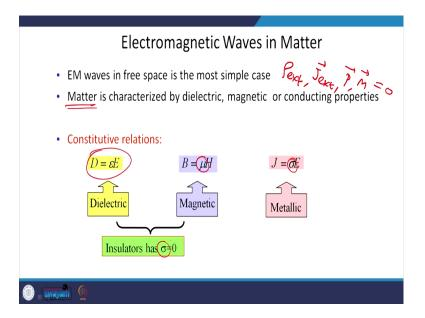
So, basically rho external, J external and P and M, this all was equal to 0 for free space, but when there is a matter, say for example, glass then we need to consider certain properties, which are either dielectric, magnetic or conducting properties.
