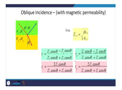
Similarly, you can solve it for s polarized light. This is what we have got here for the r p and for t p. Similarly, you can solve it for r s and t s and we see that amplitude - these are the amplitude reflection coefficients. So, you can basically calculate what is capital R and capital T.
