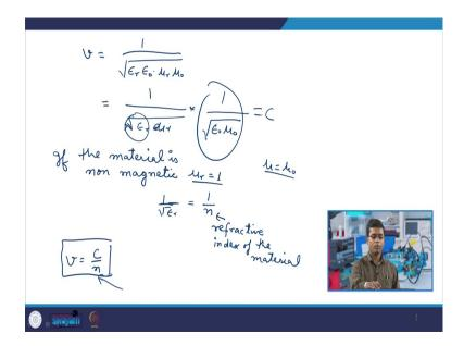
So, what you see here is that, basically, we can write v equal to 1 upon epsilon r epsilon 0 into mu r mu 0. We can take epsilon r and mu r outside. So, it becomes under root epsilon r under root mu r into 1 upon epsilon 0, mu 0, this is equal to c.
