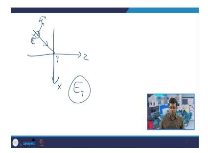
So, the electric field is now in y direction perpendicular to the plane. So, you have to solve for this wave - the electric field is here and now the magnetic field is here. H is pointing in this direction an electric field this, then you have to see what happens at the reflection and transmission. This is a homework for you.
