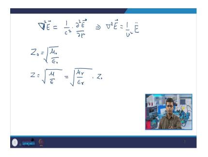
I wrote in the slightly in different form and that was del 2 E equal to 1 upon c square into del 2 E by del t square. You can write it del 2 E is equal to 1 by c square- now, in the present case it will become one by v square into E double dot ok.
