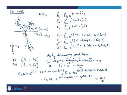
So, let us consider an interface of two media. And, we have refractive indices n 1 and n 2 for media 1 and 2 and it has also epsilon 1 mu 1, epsilon 2 mu 2 and we consider that an electromagnetic wave is incident at angle theta 1, a part of it gets refracted at angle theta 2, and other part of it gets reflected, let us say that this is angle theta 3.
