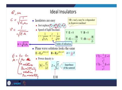
So, you take this kind of material and let us see what happens to insulators. So, in insulators, we know, that there was epsilon and mu, just replace epsilon 0 with epsilon and mu 0 with mu. So, the speed of light which we saw was c equal to one upon under root epsilon 0, mu 0.
