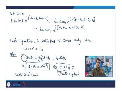
So, at x is equal to 0, E i 0 cos theta 1, that is the tangential component, into e to power i omega t minus k 1 sin theta 1 into z minus E r 0. I am removing the vector sign, because you can put it always, but let us be more simpl, that was omega dash or omega 2 omega dash let us check. So, omega dash omega dash t minus k 1 sin theta 3 into z is equal to E t 0 cos theta 2 e to power i omega 2 t minus k 2 sin theta 2 into z.
