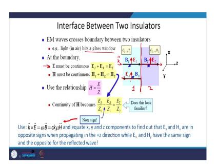
So, let us talk about an interface of two insulators. We have here an interface of two media. This is an interface. Light comes from here. So, that dielectric properties are epsilon1 and mu1 here of the first medium, epsilon 2 and mu 2 for the second medium. The k vector of the incident light is in this direction that is perpendicular to the interface.
