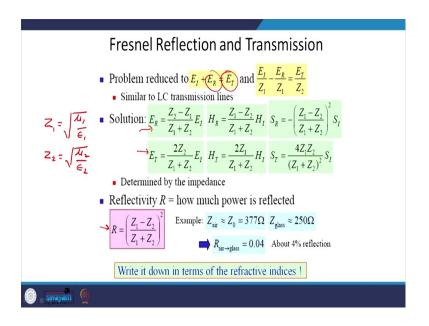
So, you solve for Fresnel reflection and transmission. Now, the problem was reduced to 2 equations in E R and E T. You have to actually calculate the ratio of E R by E I and E T by E I. And, if you solve it, you come to these equations E R E T, H R H T and S is pointing vector. So, now, you know in terms of the impedance - Z is an impedance. Z 1 is under root mu 1 by epsilon 1, Z 2 is under root mu 2 by epsilon 2, you know this.
