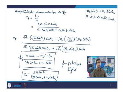
What is the amplitude transmission coefficient? Amplitude transmission coefficient, that is t p is equal to E t 0 divided by E i 0. And, you get 2 epsilon 1 sin theta 1 cos theta 1 divided by epsilon 2 sin theta 2 cos theta 1 plus epsilon 1 sin theta 1 cos theta 2. Now, as we know n 1 sin theta 1 is equal to n 2 sin theta 2 we can write in it in terms of n.
