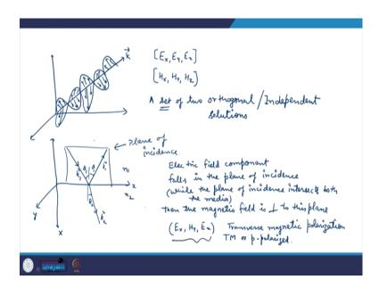
So, suppose we have an electromagnetic wave which is going in an arbitrary direction and the k vector defines the direction of propagation of the wave. The electric field oscillations are like this, and the magnetic field oscillations will be in the perpendicular directions. So, it will be like this, something like this. So, what you see is that if you want to know the electric field and magnetic field in an electromagnetic wave you have to solve for 6 components E x, E y, E z and H x, H y, H z.
