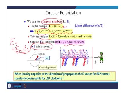
And not only that we can do more also, how? Take a complex number. So, rather writing E 0 as a real function, you can write it E 0, i E 0. What it means here? It means that, now it has 2 components and they have a phase difference of pi by 2 - 90 degrees phase difference. You write the wave equation for a plane wave and you resolve it in 2 components, the real part and the imaginary part.
