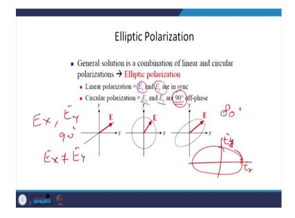
Circular polarization is a special case of elliptical polarization and similarly linear polarization is also a particular case of elliptical polarization. So, you see, that in linear polarization E x and E y are in synchronization. In circular polarization they are 90 degree off phase, but if they are not 90 degree, say they are 80 degree only, what will happen?
