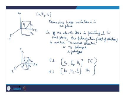
Similarly, one can have another. So, this was your structure - you had y here, you had z and x here. So, you can have H x, E y, H z. Again, the reflective index variation is in x z plane. So, if the electric field is pointing perpendicular to the interface - this plane, the polarization is called, polarization means actually the set of solution, set of solution; I told you about 2 independent set of solutions, this is called Transverse Electric or T E polarized or you can say s polarized.
