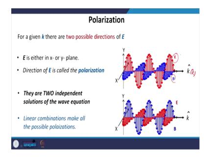
So, suppose this k is propagating in this Z direction so, the way this propagating in Z direction. So, E can be either in x plane or y plane. You can see here the blue ones are magnetic field E is red ones are electric field. So, it is in y plane or in x plane.
