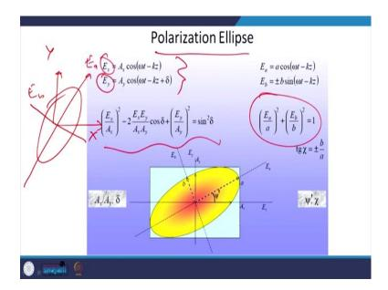
Suppose I have a random elliptical polarization like this. And, if I have a component where I want to measure how much ellipticity it has? what is the direction of polarization? if it is a right circular left right elliptical or left elliptical?, then what we need to do is that we have x and y axis. And, for E x and E y we can write these equations.
