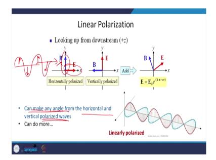
So, if you see for linear polarization, let us say that the wave is going in plus z direction and we see from bottom what will we see? We will see an electric and magnetic field vectors. Basically, it is wave - it is a variation of electric field like this in x direction & magnetic field in y, but what you are actually see is like vectors. You do not see this oscillation, because it is happening in the same plane.
