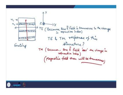
Now, suppose I have a structure made on glass, which has this kind of variation of refractive index. Suppose this region has refractive index n 1, this region has refractive index n 2 and this is periodic, and light is incident from the top. So, you have, suppose, x, y, z like this. So, z is the direction of propagation. You can think like this. Suppose, z is pointing down to the plane.
