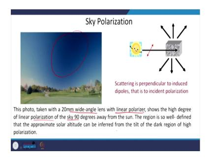
Sky polarization: So, scattering is perpendicular to induced dipoles and that is to incident polarization. So, if you change the polarization, basically you see different orientation of it and different scattered light. So, this photo was taken with a 20 mili- meter wide angle lens with a linear polarizer. And, see high degree of linear polarization of the sky 90 degrees away from the sun. You can see here darker patch.
