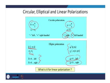
So, if you have elliptical polarizations or say circular polarization delta is equal to plus pi by 2 or minus pi by 2 and you can have psi like this and a must be equal to b. So, if this is negative right circularly polarized you have positive then left circularly polarized and vice versa, same here.
