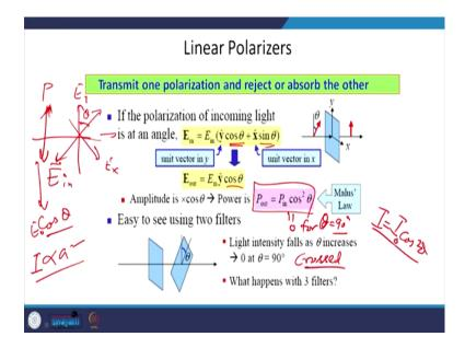
What is the linear polarization? It transmits one polarization - rejects or absorbs the other. Let us come back to that virtual experiment which I told you -that you tie a rope and I am swinging it like this. What I do is that, now I put a chair, which has openings like this. And, I am swinging like this -what will happen? It will not stop the oscillations like this in this plane. So, it is letting it pass through.
