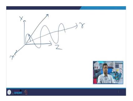
So, suppose you have x y z and you can have a wave which is travelling in this direction r, then it will have electric field components in all the x y z coordinates. You can resolve it in two orthogonal polarizations; we will come to that. And, any other configuration will be a combination of these two independent solutions.
