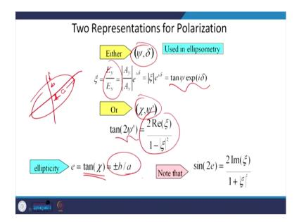
There are two representations for polarization: this one is used in ellipsometry, where you define psi like this zeta and solve for this; or you have this representation, where you take tan 2 psi 0 is equal to this. You define the ellipticity equal to tan of psi - this angle, that comes from b by a. You remember this? When it was ellipse? The minor one is b, major one is a, and you have this ellipse as b by a.
