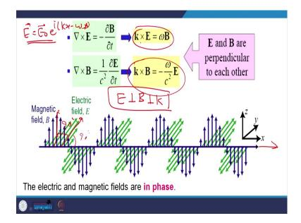
If you put this E is equal to E 0 e to power i k x minus omega t, this equation, you end up with this relation. And the 4th equation you end up with this relation. What these two say? - these two say that E and B are perpendicular to each other. So, from here it seems that E is perpendicular to B and perpendicular to k. So, they are all mutually orthogonal triads.
