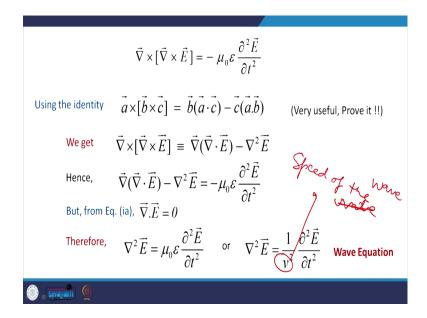
v is the speed of the wave. So, this relation is called a wave equation.
