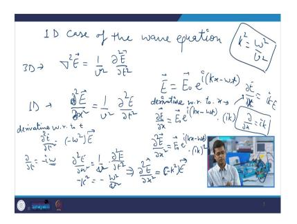
So, if you write a one-dimensional case of the wave equation that will be. So, wave equation was I mean 3D, 3D it was del 2 E is equal to 1 by v square del 2 E by del t square. Now, if you take 1D case it will become d 2 E by d x square del 2 E by d x square is equal to 1 by v square del 2 E by del t square I mean it has to be partial derivative.
