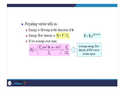
Poynting vector tells us that energy is flowing in the direction of propagation of the wave that is the vector k, and the energy flow density is E square by Z naught. So, if we average over time you get by a factor of half because you have a cos square term, average of which comes out to be 1 by 2. So, average energy flow density of E m waves in free space is E 0 square by 2 Z 0.
